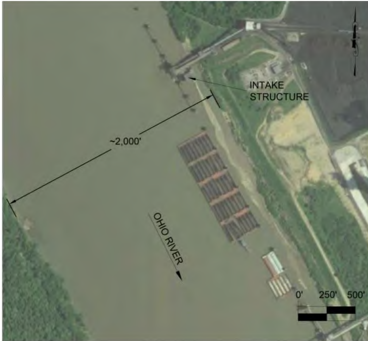
Figure 2-3 River Width Near Trimble County
