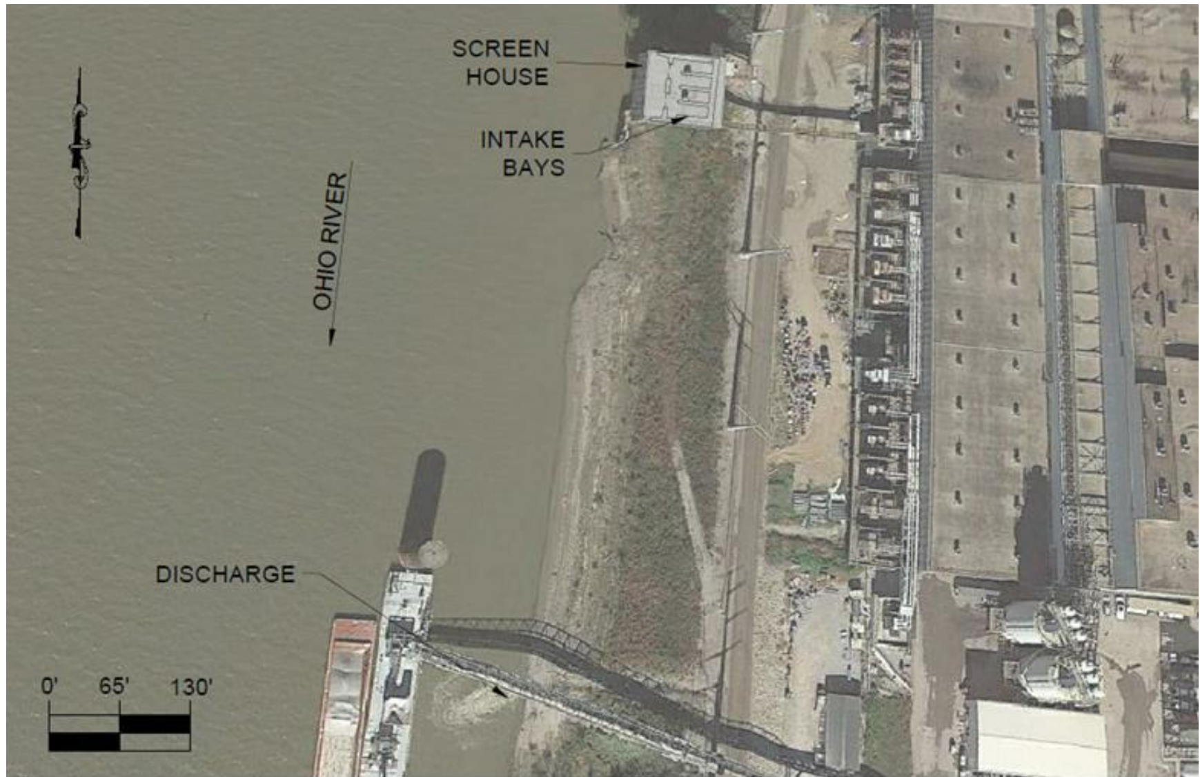
Figure 3-2 Mill Creek CWIS Configuration
