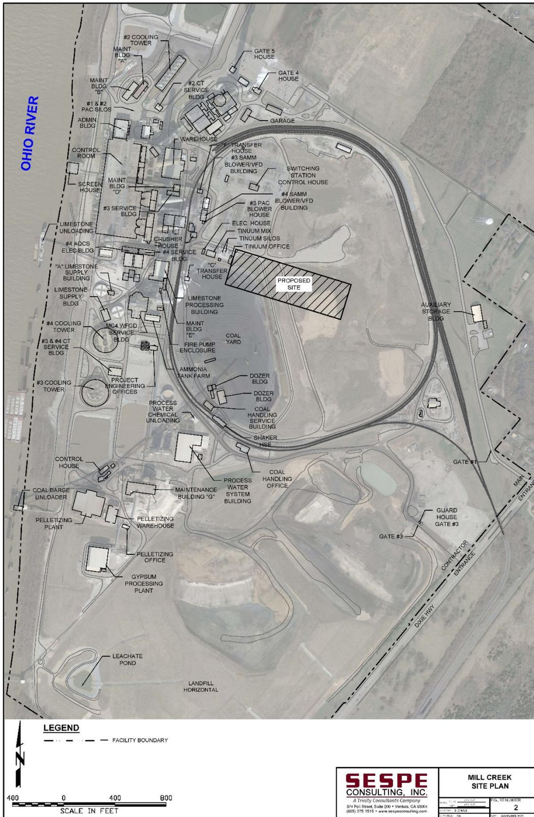
Figure 3. Proposed NGCC Unit Installation Components, Infrastructure Connections and Setback
