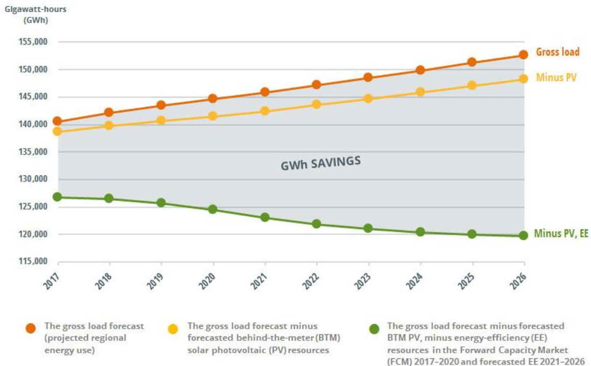
Figure 2. Projected annual energy use in ISO NE with and without energy efficiency. Source: ISO NE 2018a.
