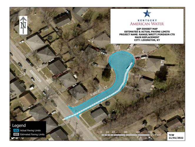
The estimated amount of paving required for the Range/Writt/Fordson project was initially 5,600 square feet compared to the final amount of 15,085 square feet. The estimated cost was initially \$46,603.20 compared to the final cost of \$147,051.84.
