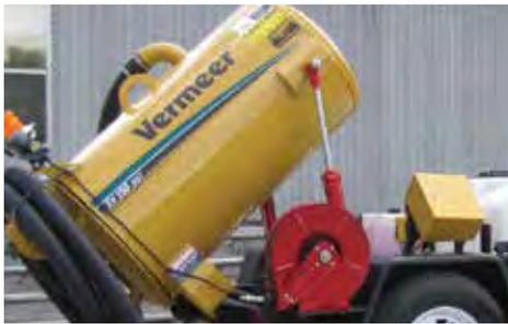
**HYDRAULIC TILT TANK.** Efficiently offload debris.
