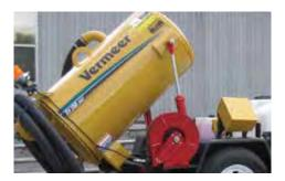
HYDRAULIC TILT TANK. Efficiently offload debris.
