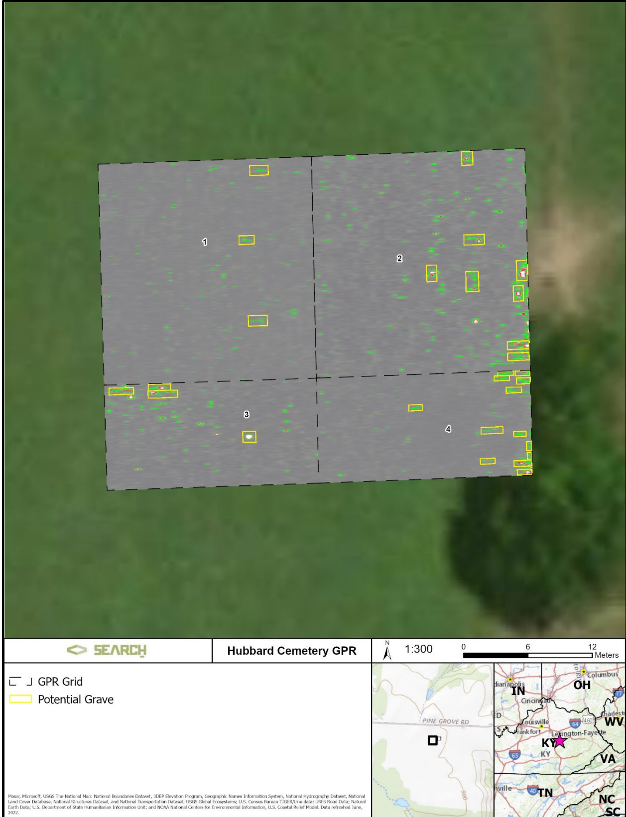
Figure 5. RADAN 7 time slice results with anomalies consistent with graves indicated.
