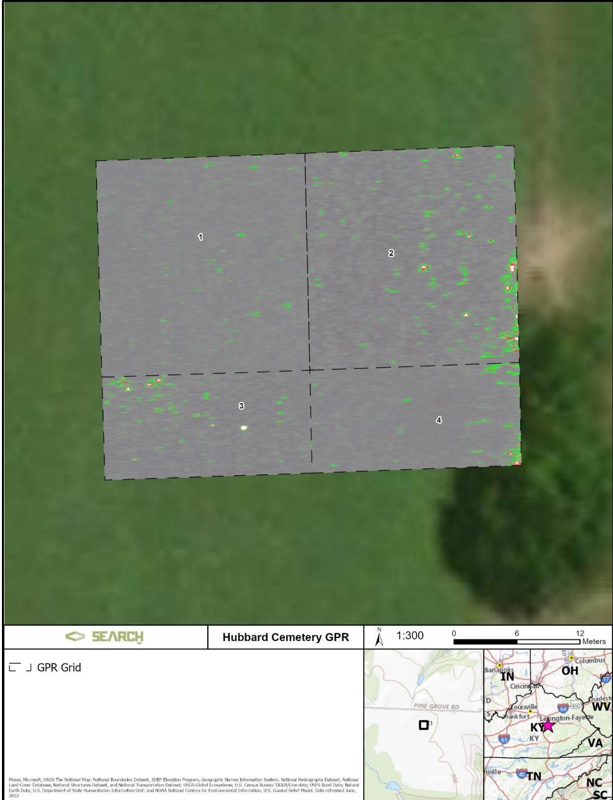
Figure 4. RADAN 7 time slice results showing anomalies between 30 to 125 cmbs (1 to 4 ftbs).
