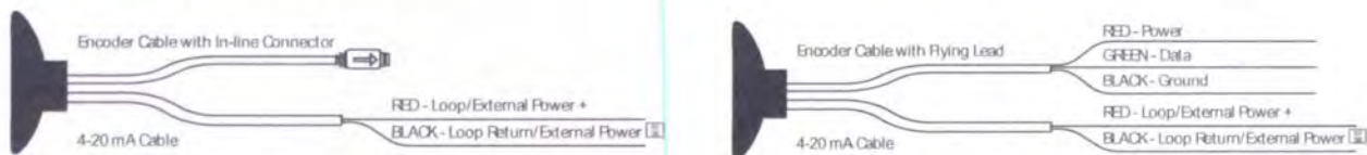
Figure 3: HR-E LCD 4-20 wiring options
