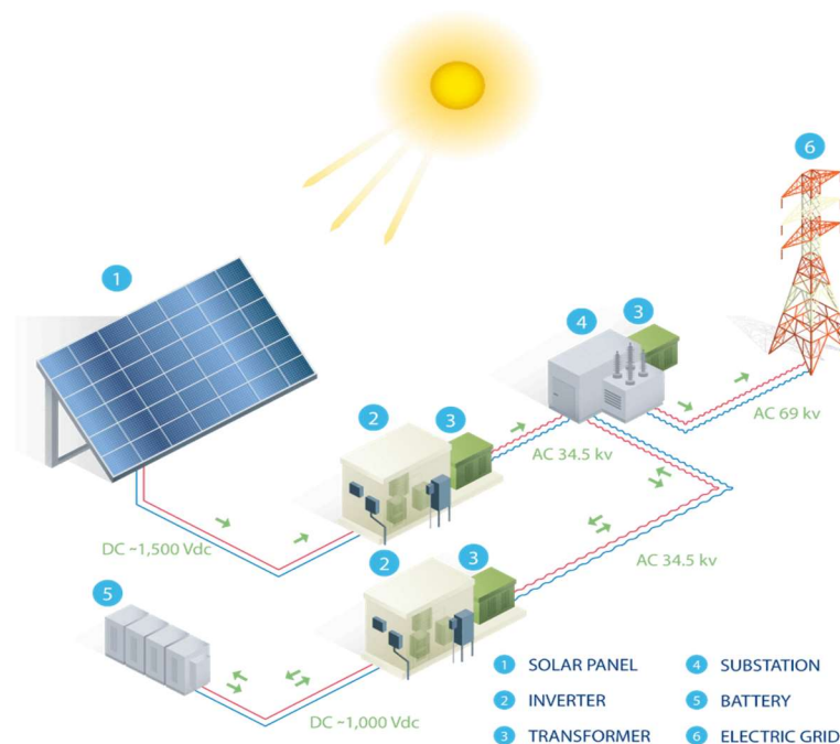
Figure (2) A Solar Power Plant 2
