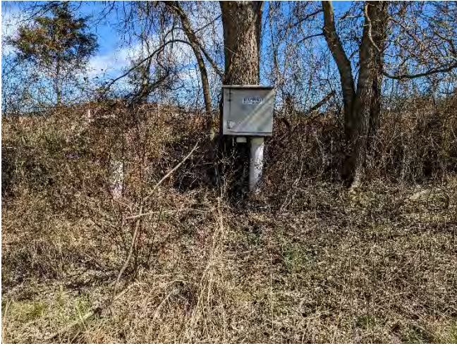
Photo 7: Groundwater monitoring well
