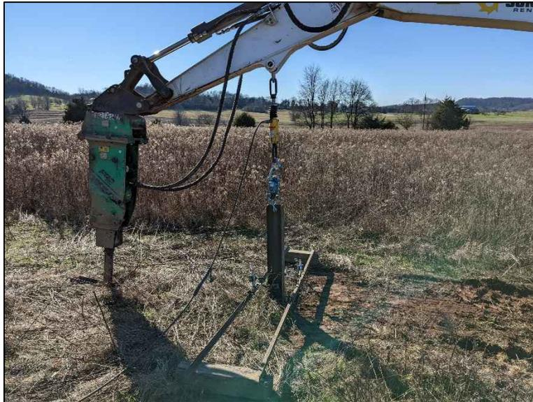
*Pile Tension Load Test Setup*
