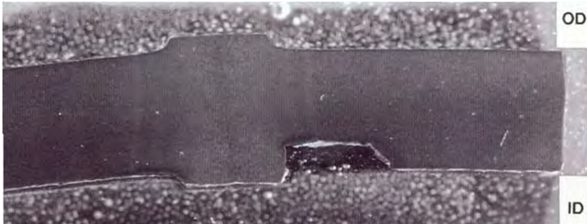
Photographs of Weld Seam ID Surface and Metallographic Section.
