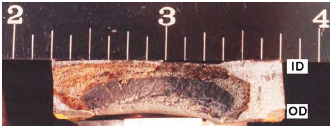
Photographs/Micrographs of Weld Seam OD Surface and Fracture Surface.
