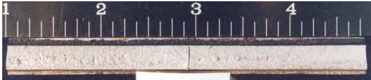
Photographs of Weld Seam ID Surface and Fracture Surface.
