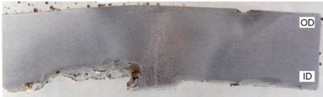
Photographs of Weld Seam ID Surface and Metallographic Section.
