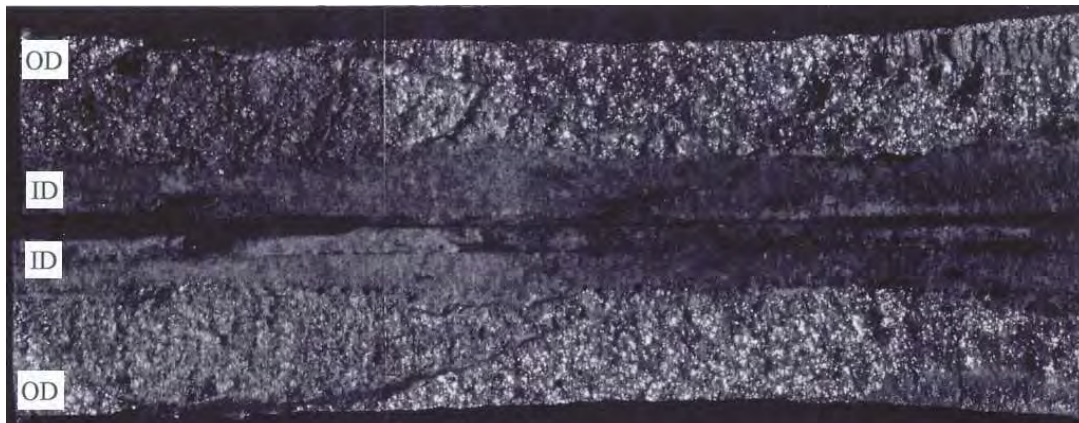
Photographs of Pipe Seam ID Surface and Fracture Surfaces.
