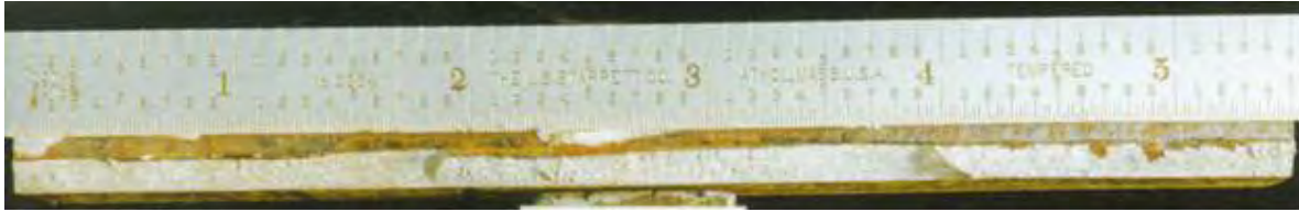
Photograph of Fracture Surface.
