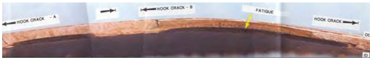
Photograph of Fracture Surface.
