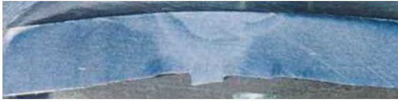
Photograph of Metallographic Section.
