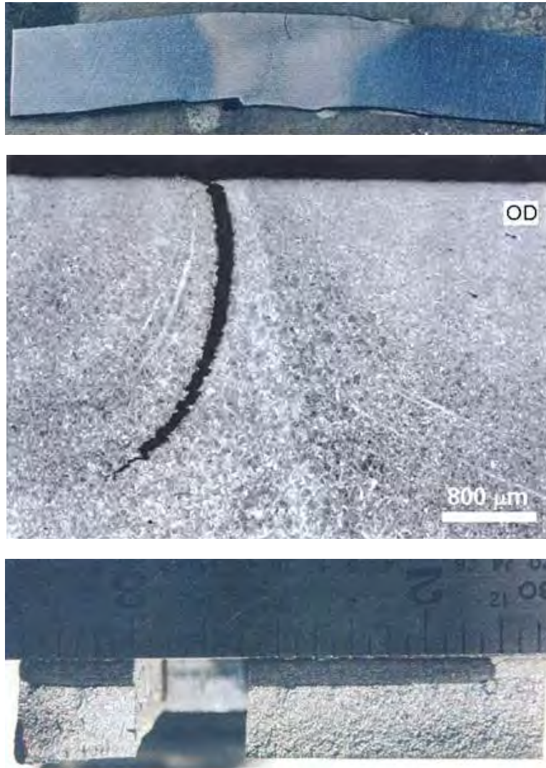
Photographs and Photomicrograph of Metallographic Section and Fracture Surface.
