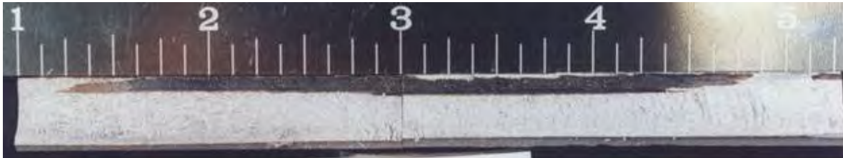
Photographs of Weld Seam ID Surface and Fracture Surface.
