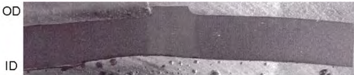
Photographs of Weld Seam ID Surface and Metallographic Section.
