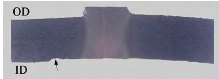
Photographs of Weld Seam ID Surface and Metallographic Section.
