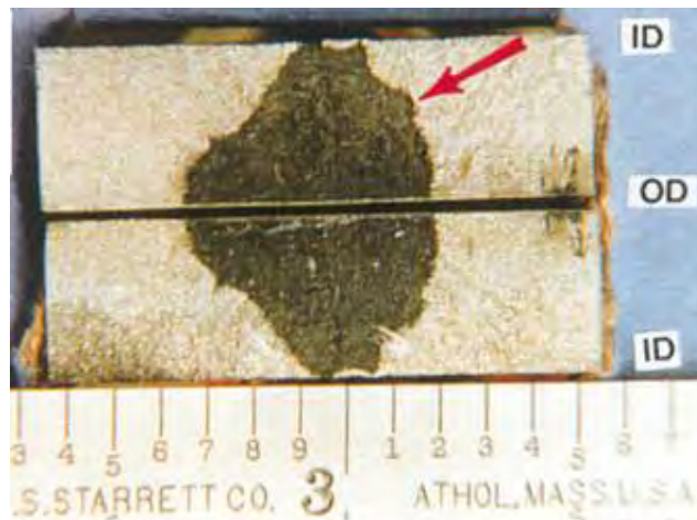
Photograph of Magnetic Particle Indication on Pipe OD Surface and of Fracture Surfaces.
