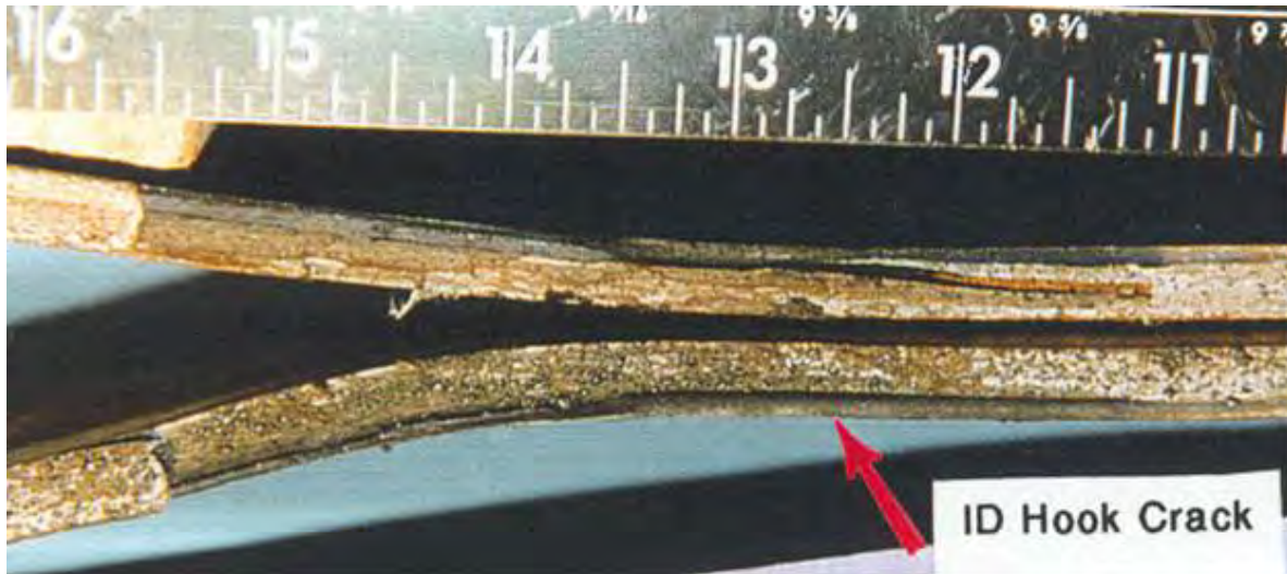
Photograph of Fracture Surfaces.
