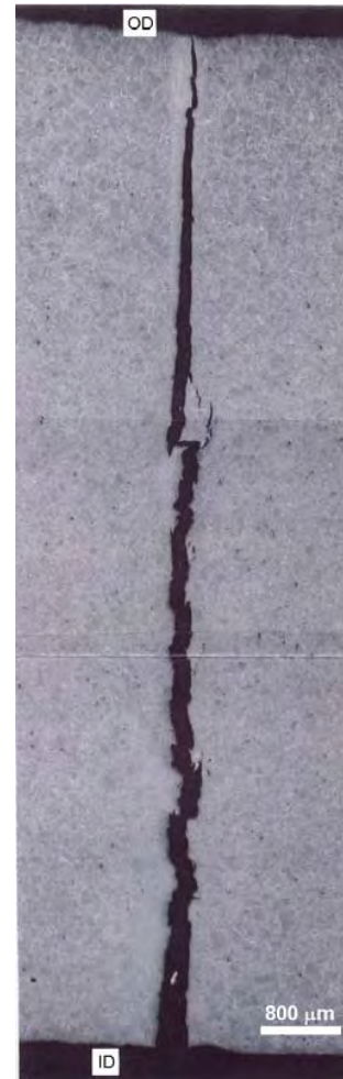
Photographs and Photomicrograph of Metallographic Section and Fracture Surfaces.
