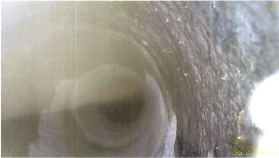
View of limestone with dark staining at -33'.
