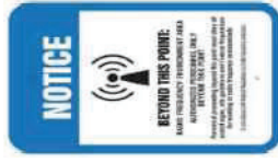
2 1 NOTICE RF SIGN (BLUE) WHITE BACKGROUND, WHITE LETTERING MOUNTING LOCATION: GATE & CENTERLINE OF FENCING AROUND SITE (QTY: 4) WHERE ACCESS GATE INSTALLED (QTY: 5)
