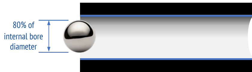
A steel ball is used to 'prove' the integrity of the internal bore
