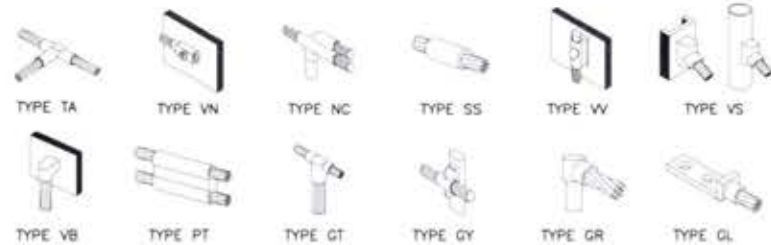
1 CADWELD GROUNDING CONNECTION DETAILS NOT TO SCALE
