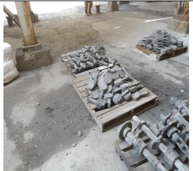
Top Left: Another example of missing collecting plate hammers along with broken shock bars in the same area. Top Right: A pallet of replacement hammers for the ESPs. A few different hammer bracket styles are being used in the unit. Bottom Left: A photo of a broken high voltage rapper rod. This rod was touching the high voltage from the field beside it. Bottom Right: A photo of a broken high voltage lifting rod.
