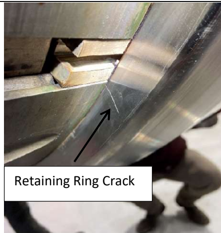
AS FOUND EXCITER END RETAINING RING CRACK WITH DYE PENETRANT
