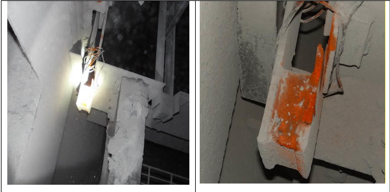
Top Left and Right: A photo of tie wire holding collecting plate shock bars together. This is a poor repair. Shock bars need to be either repaired properly or the entire shock bar should be changed. Bottom Left: A photo of a shock bar that has come out of the plate guide. Bottom Right: More examples of holes found in the collecting plates.
