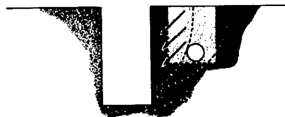
Figure 31-5: Unstable Soil Near Old Trenches
