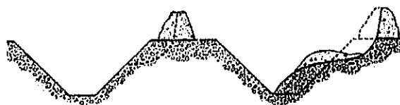
Figure 31-11: Angle of Sloping Must Support Spoil Piles
