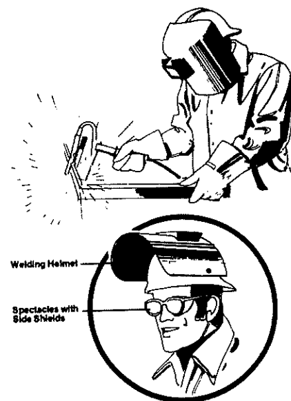
Figure 11-16: Protection from Injurious Radiation (Electric Arc Welding)
