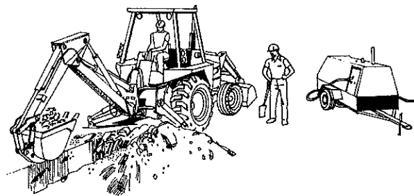
If a backhoe and a compressor each produce 90 dB of noise, the worker standing between them is exposed to 93 dB, which is double the amount of noise intensity.
