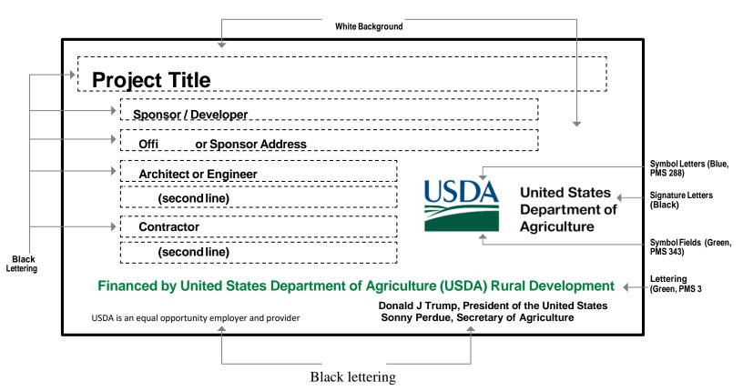
Sign Dimensions: 1200 mm x 2400 mm x 19 mm (approx. 4' x 8' x <sup>3</sup>/<sub>4</sub>") PLYWOOD PANEL (APA RATED A-B GRADE–EXTERIOR)
