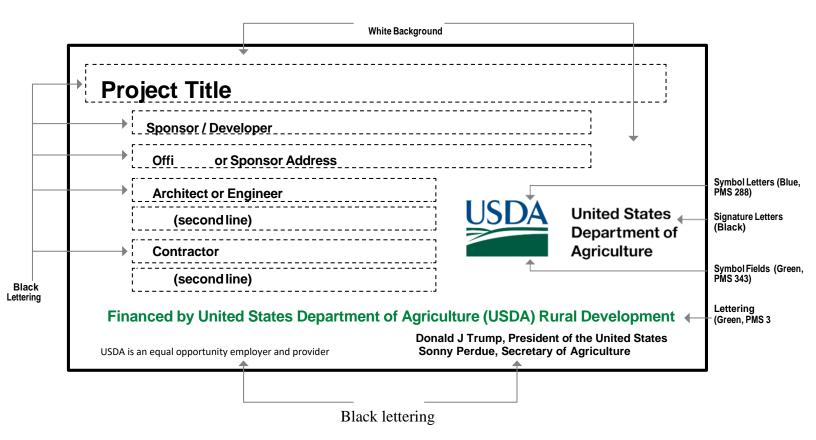
Sign Dimensions:  $1200 \text{ mm x } 2400 \text{ mm x } 19 \text{ mm (approx. 4' x 8' x <math>^{3}4$ ")} PLYWOOD PANEL (APA RATED A-B GRADE-EXTERIOR)
