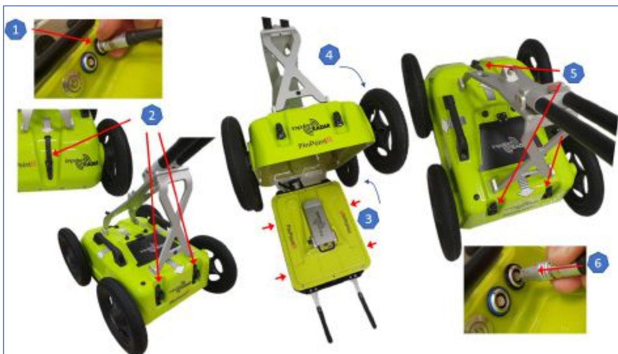
Figure 6 GPR unit fitting and height adjustments
