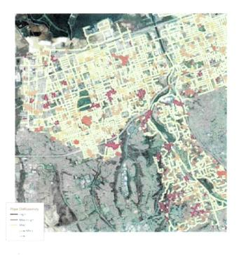
ASTERRA MasterPlan's key "deliverable" is a GIS dataset containing pipe deficiency levels derived from SAR data. This product is based on the same proven patented algorithm that is used by Recover to detect leaks in your system but is extended to monitor your system over time using statistical analysis.
