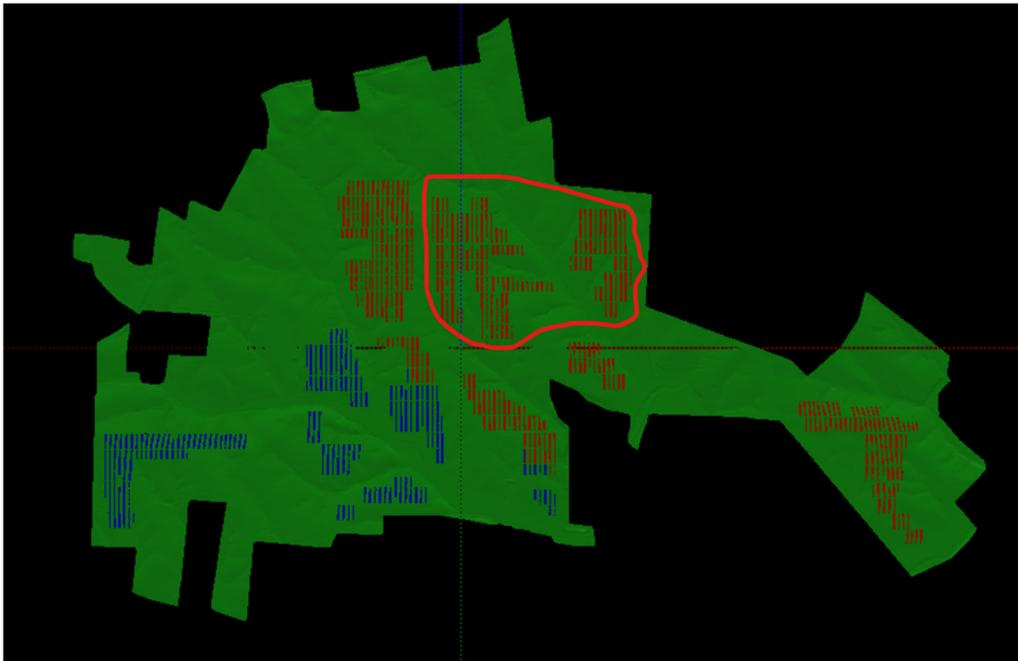
*Trackers causing potential reflectivity events at KOP R20. Visible trackers enclosed in red shape.*
