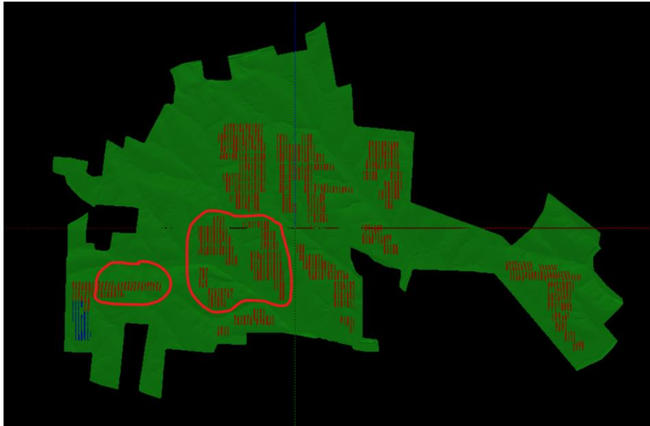
*Trackers causing potential reflectivity events at KOP R15. Visible trackers enclosed in red shape.*
