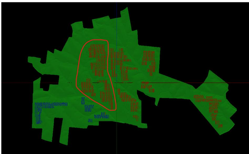
*Trackers causing potential reflectivity events at KOPs R17, R18 & R19. Visible trackers enclosed in red shape.*
