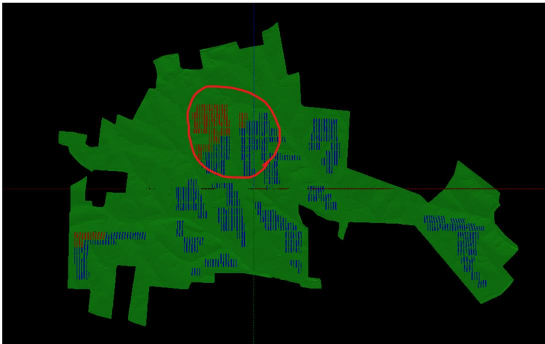
*Trackers causing potential reflectivity events at KOPs R25 & R26. Visible trackers enclosed in red shape.*
