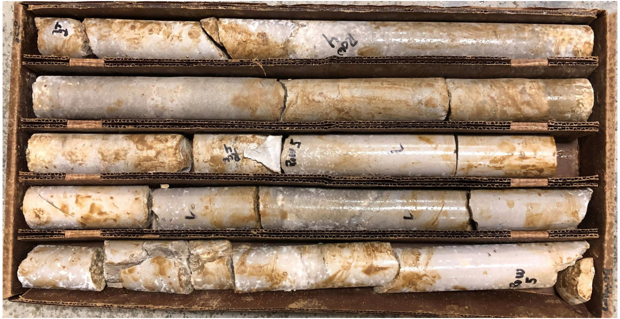
ROW-4 - Rock Core Run 1 – 18 to 23 feet ROW-5 - Rock Core Run 1 – 10 to 15 feet
