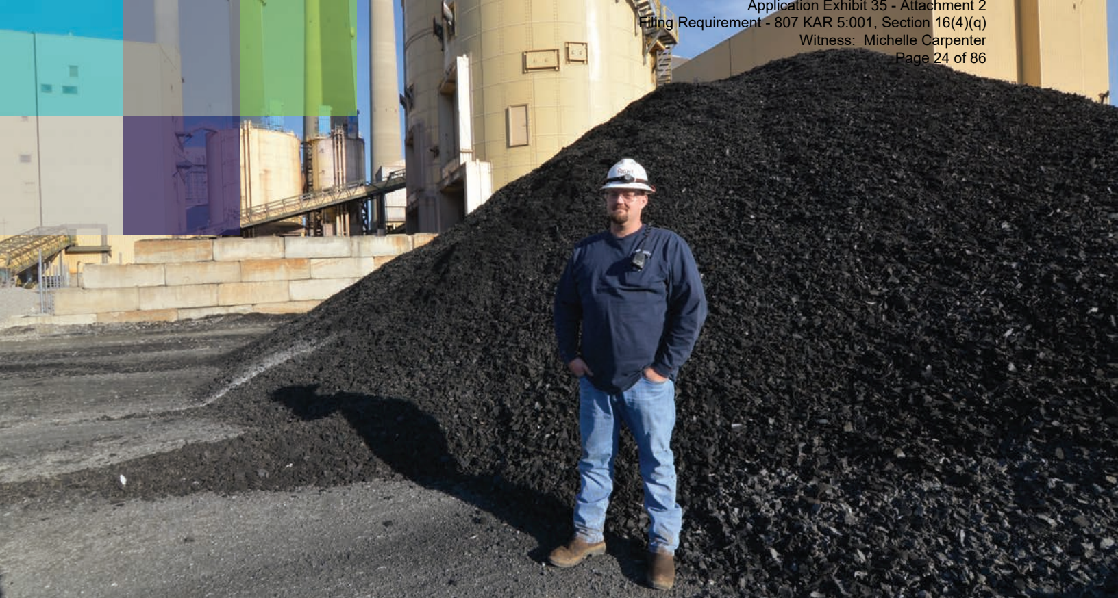
Matt Robinson stands in front of the stockpile of tire-derived fuel (TDF), which consists of tires that have been cut up for use as a supplemental fuel at Spurlock Station.
