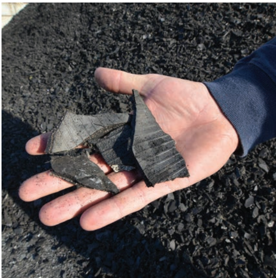
An employee holds small chunks of TDF at Spurlock Station. The plant uses the equivalent of about 2.4 million tires a year by adding TDF as fuel to generate power. That's about half of all waste tires produced in Kentucky each year.
