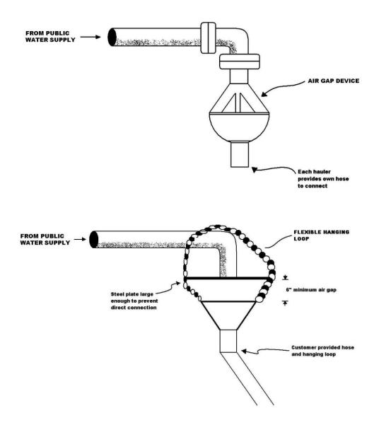
FIGURE 1 – SUGGESTED FILLING DEVICE FOR WATER LOADING STATIONS
