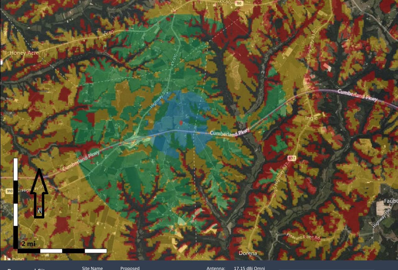
Proposed Site 1900 MHz Coverage Site Name Latitude: Longitude: Proposed N37.090347 W84.912169 Antenna: 17.15 dBi Omni
