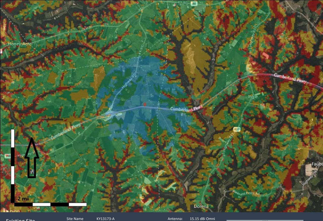
Existing Site 700 MHz Coverage Site Name Latitude: Longitude: KY13173-A N37.088828 W84.913139 Antenna: 15.15 dBi Om Alpha Rad Center (ft): 300 Azimuth (Deg): 0 ERP per RS (W): 2.0
