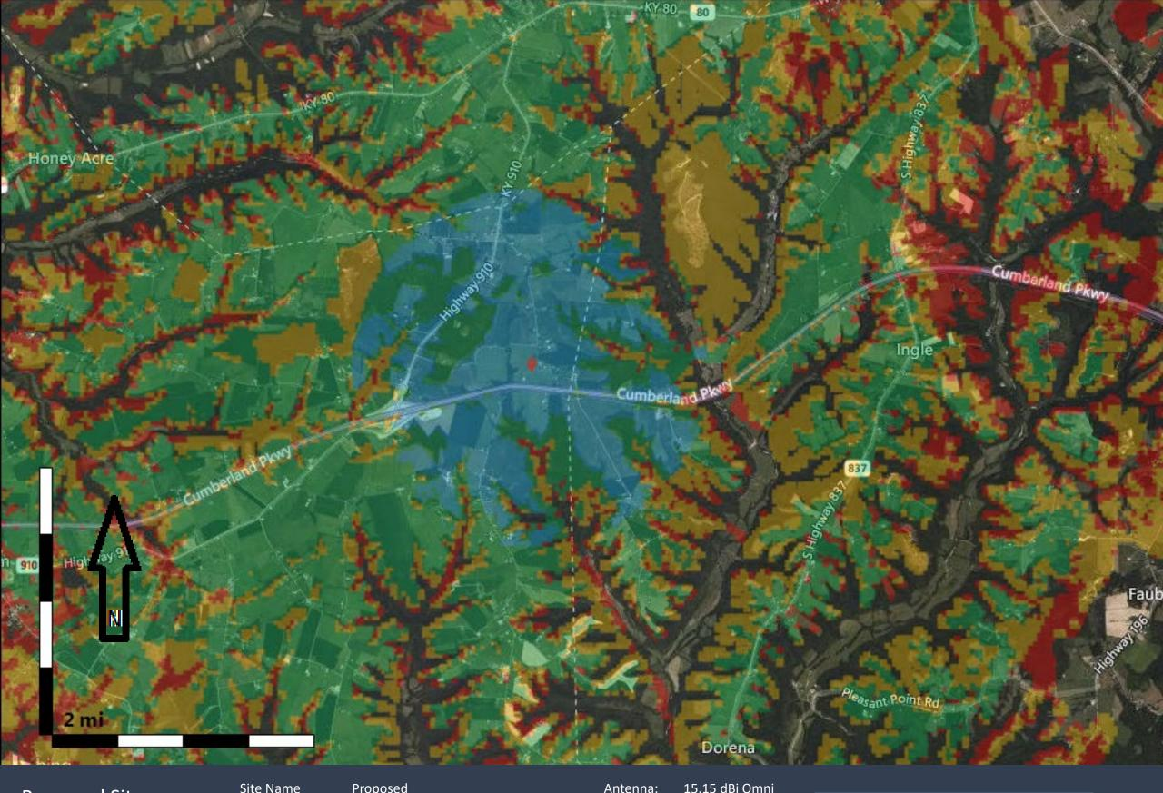
Proposed Site 700 MHz Coverage Site Name Latitude: Longitude: Proposed N37.090347 W84.912169 Antenna: 15.15 dBi Omni
