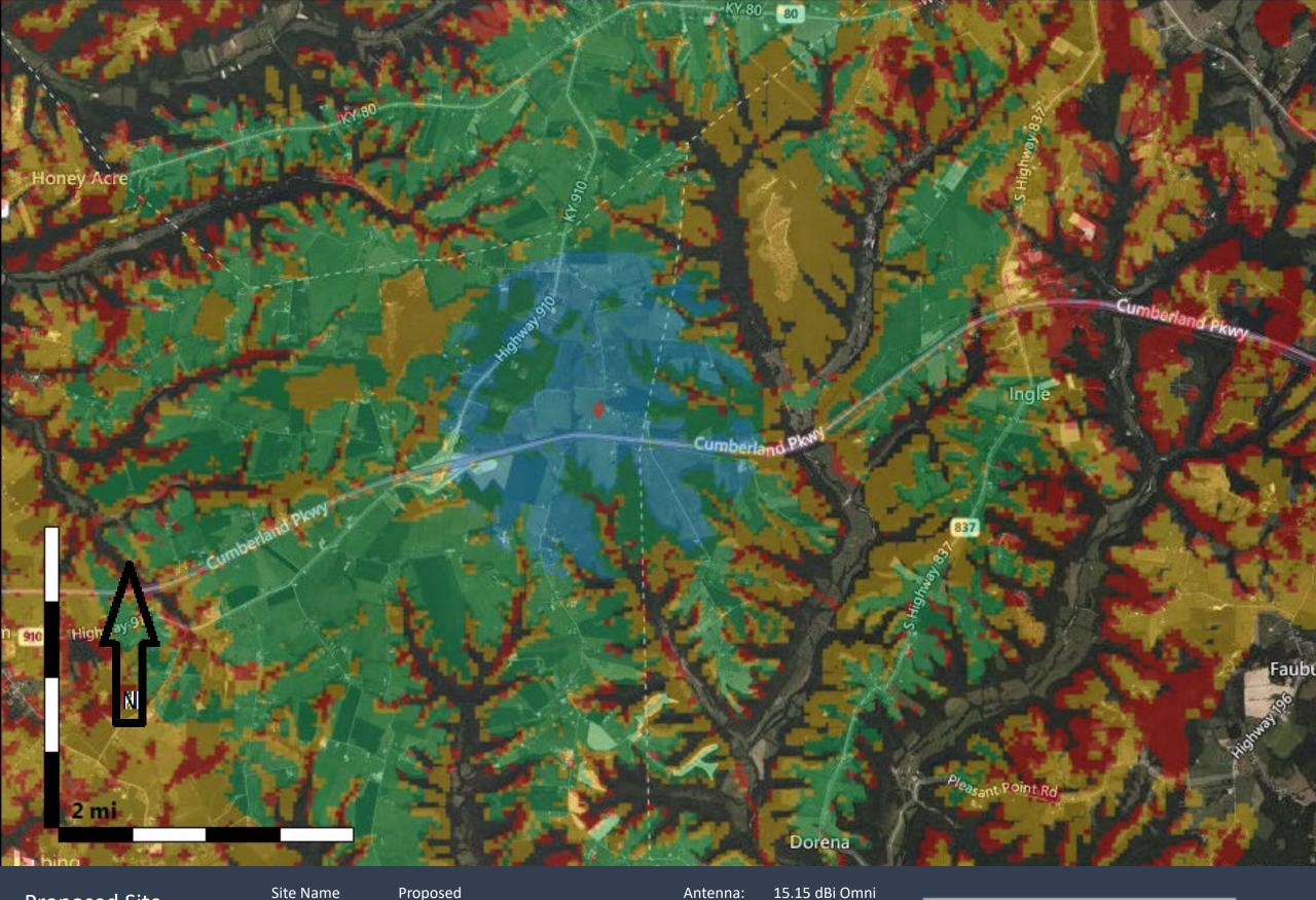
Proposed Site 850 MHz Coverage Site Name Latitude: Longitude: Proposed N37.090347 W84.912169 Antenna: 15
