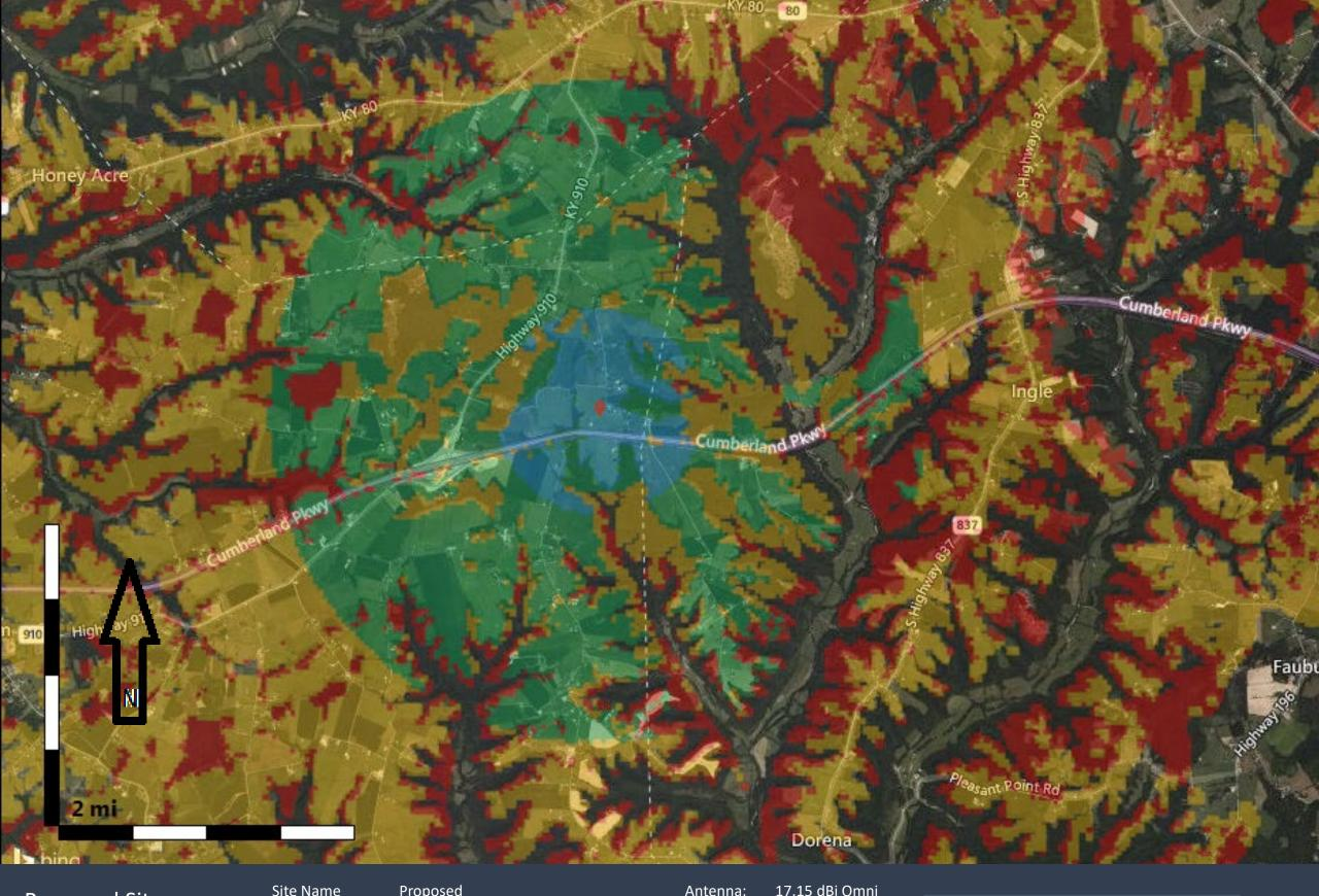
Proposed Site 2100 MHz Coverage Site Name Latitude: Longitude: Proposed N37.090347 W84.912169 Antenna: 17.15 dBi Omni
