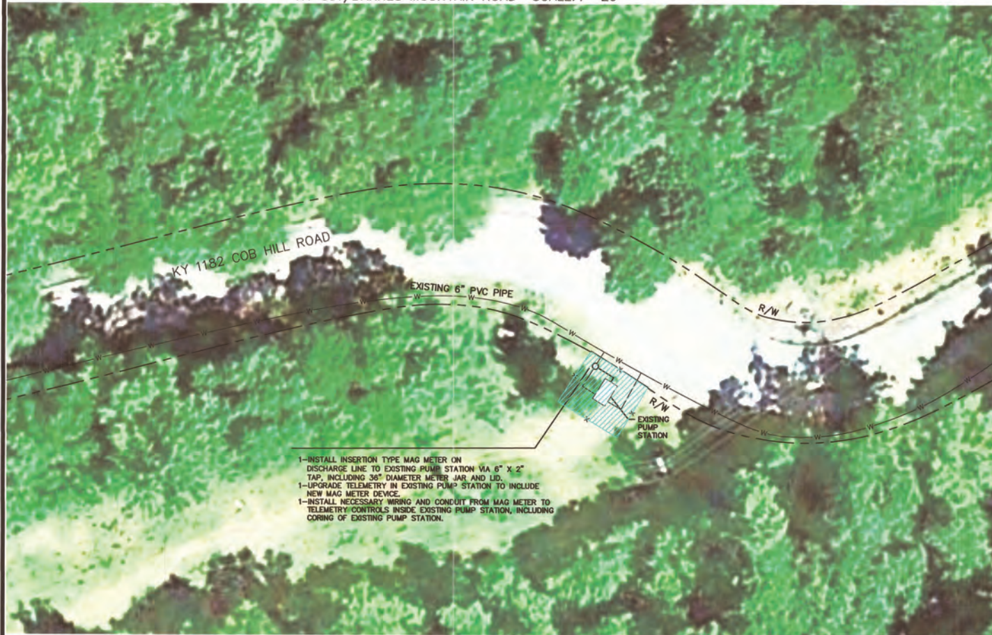
KY 1182 (COB HILL PUMP STATION) SCALE: 1"=20'
