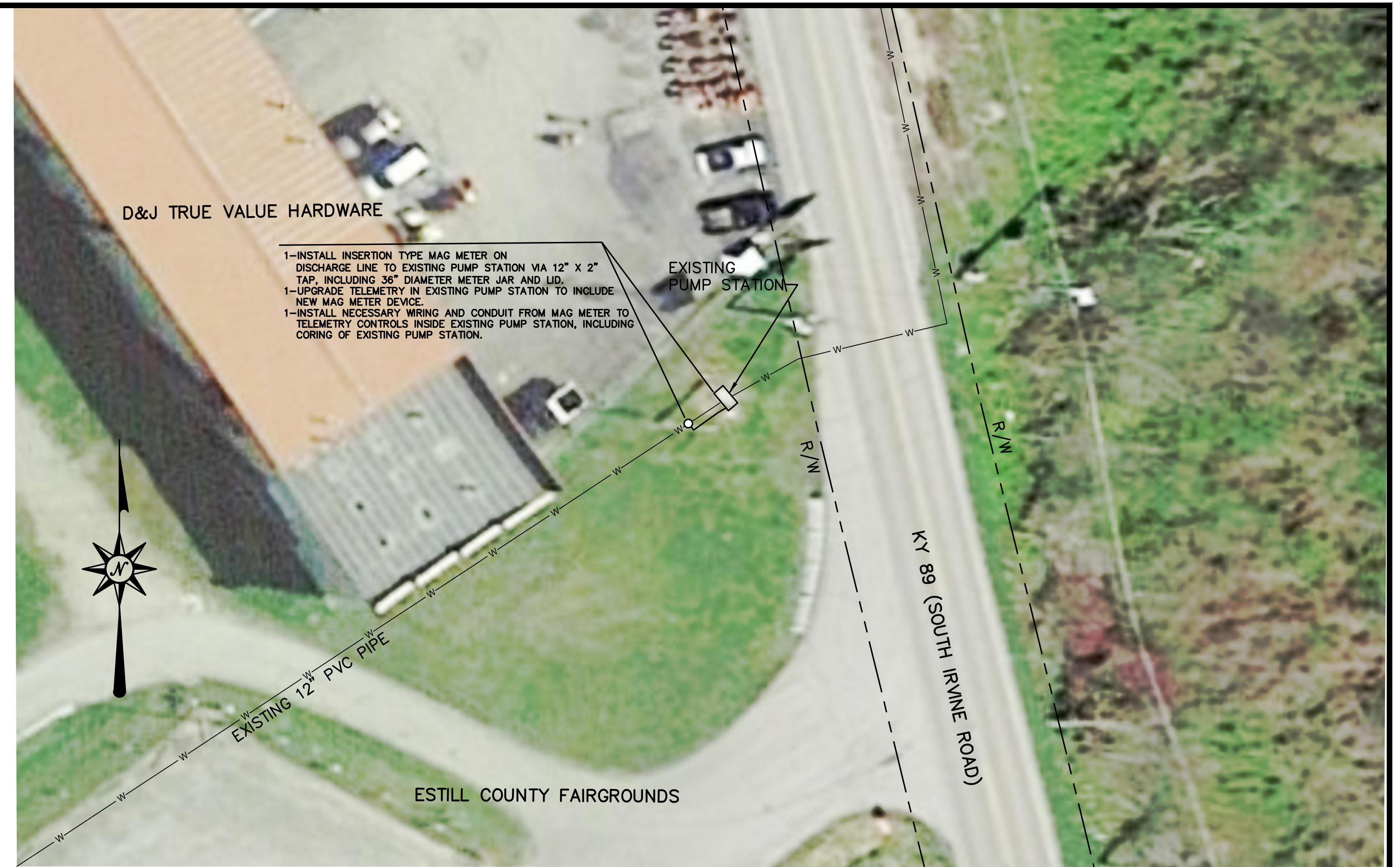
KY 89 (NEW RIVER PUMP STATION) SCALE: 1"=20'
