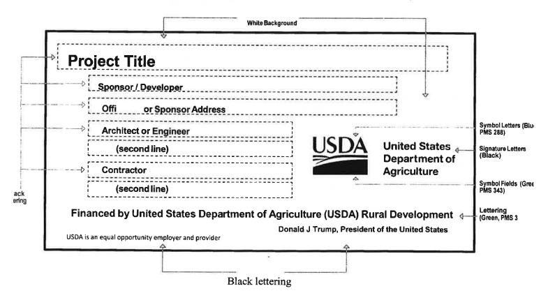
Sign Dimensions: 1200 mm x 2400 mm x 19 mm (approx. 4' x 8' x 34") PLYWOOD PANEL (APA RATED A-B GRADE-EXTERIOR)
