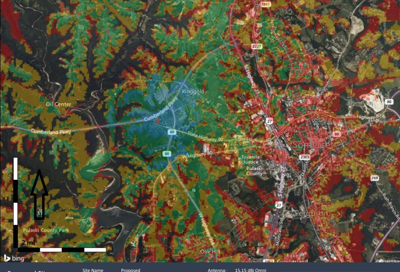
Proposed Site 850 MHz Coverage Site Name Latitude: Longitude: Proposed N37.099531 W84.667347 Antenna: 15.15 dBi Omni
