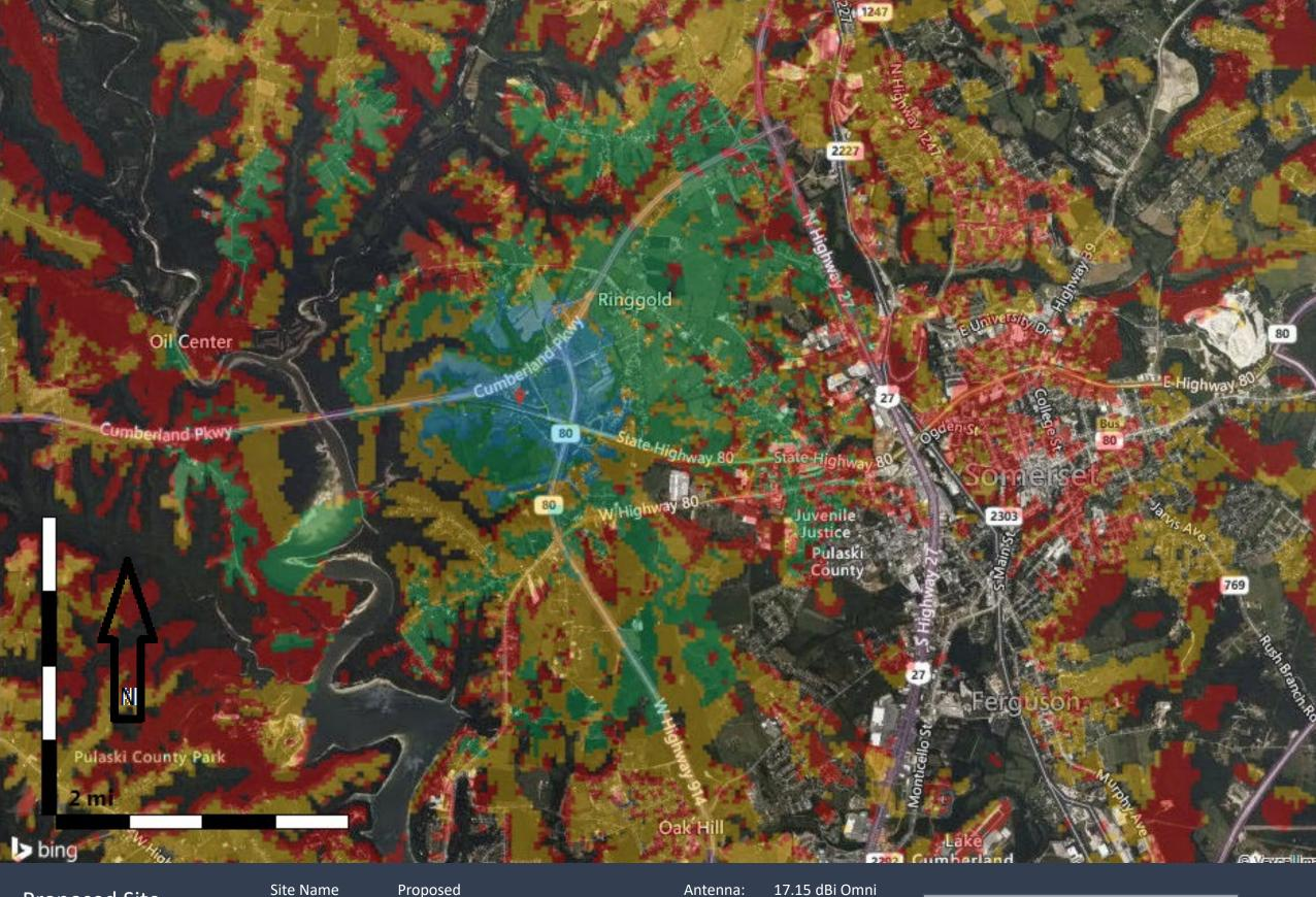
Proposed Site 1900 MHz Coverage Site Name Latitude: Longitude: Proposed N37.099531 W84.667347 Antenna: 17.15 dBi Omr Alpha Rad Center (ft): 250 Azimuth (Deg): 0 ERP per RS (W): 4.7
