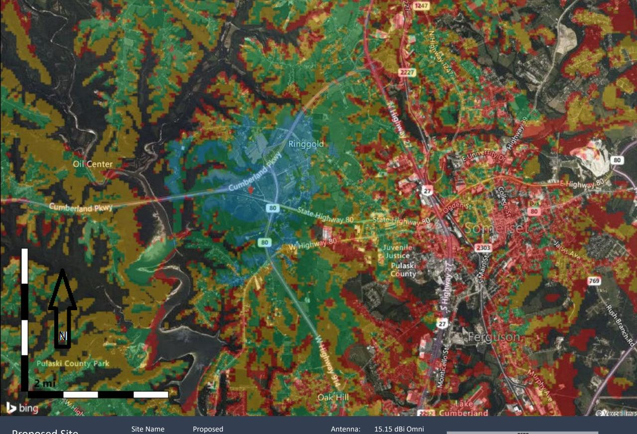
Proposed Site 700 MHz Coverage Site Name Latitude: Longitude: Proposed N37.099531 W84.667347 Antenna: 15.15 dBi Omni Alpha Rad Center (ft): 250 Azimuth (Deg): 0 ERP per RS (W): 2.0
