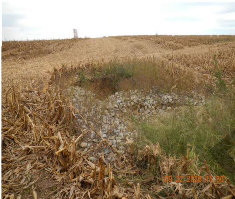
Figure 10: View of feature F-70, reopened throat that was one filled with soil and rock.
