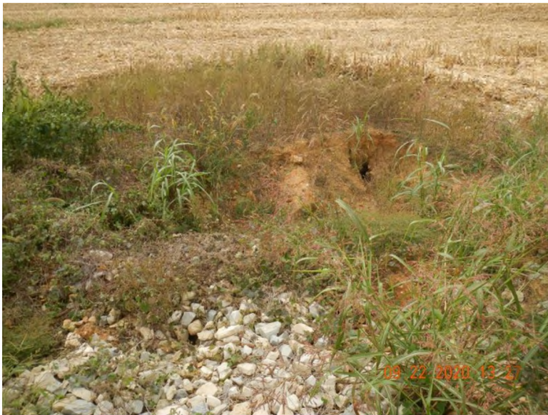
Figure 3: View of feature F-73, reopened throat that was one filled with soil and rock.
