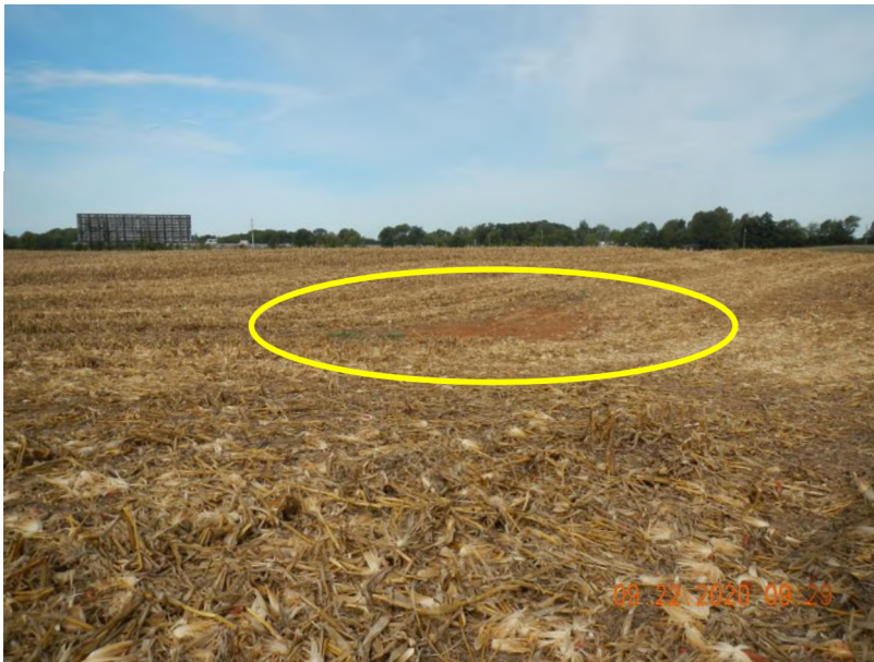
Figure 15: View of feature F-58, small, gently sloped cover subsidence with an apparent fresh soil and gravel filled open throat.
