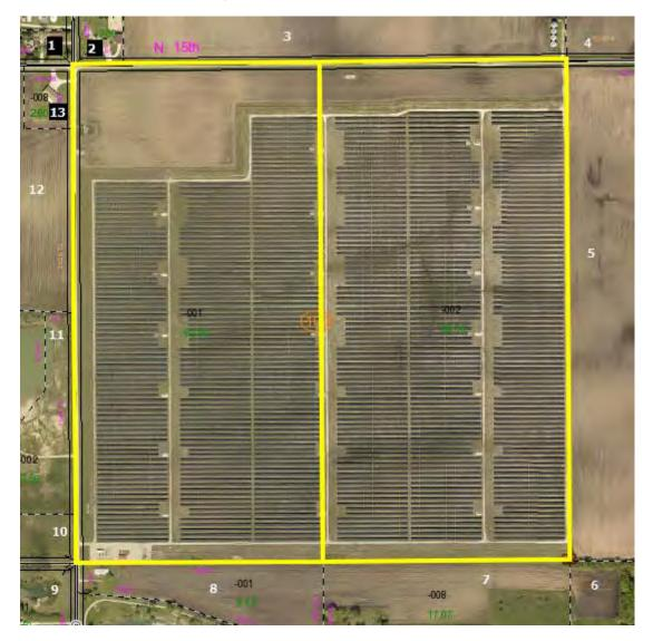
This solar farm has a 20 MW output and is located on a 160-acre tract. The project was built in 2012.
