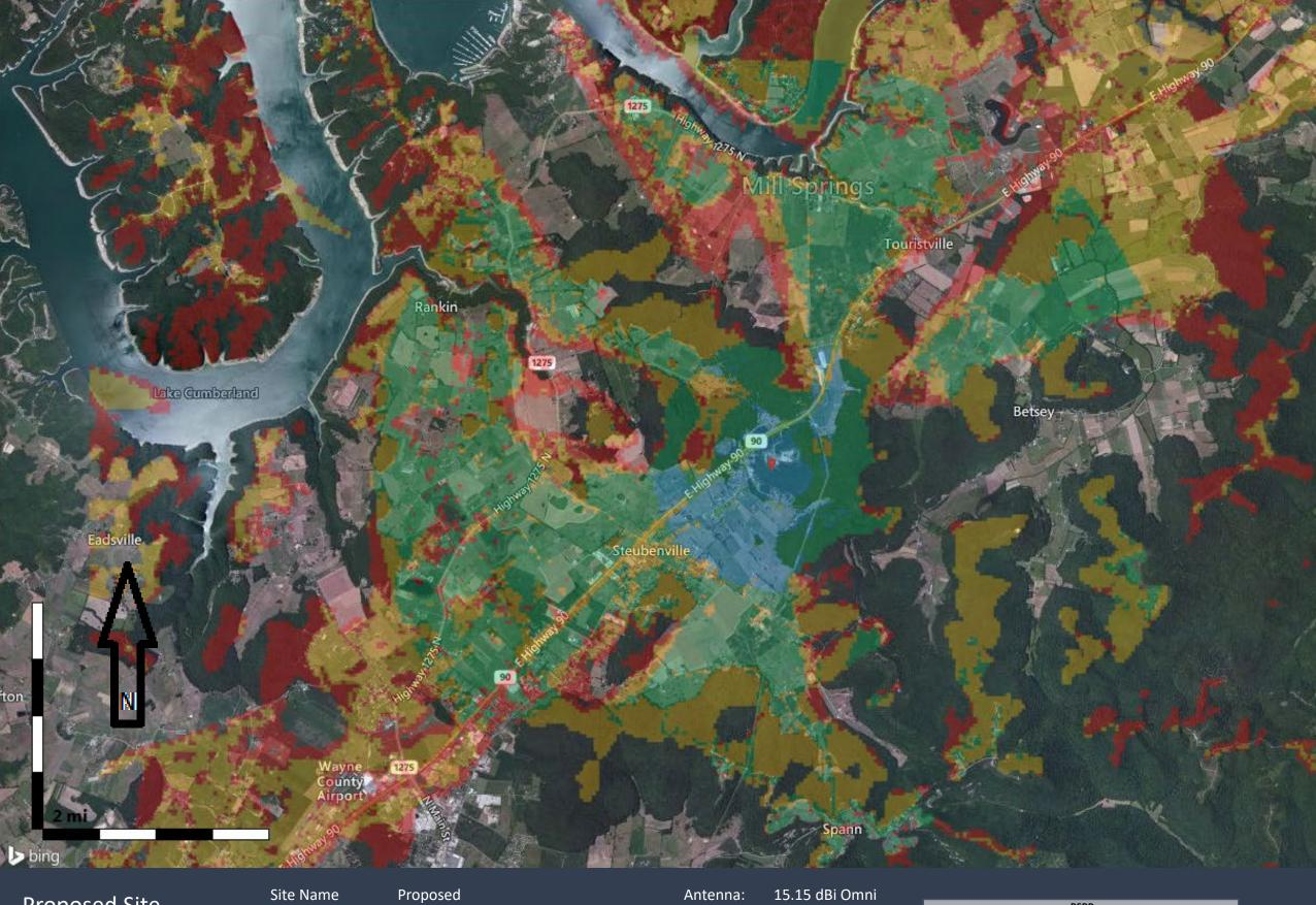
Proposed Site 850 MHz Coverage Site Name Latitude: Longitude: Proposed N36.897583 W84.784972 Antenna: 15.15 dBi Omi Alpha Rad Center (ft): 250 Azimuth (Deg): 0 ERP per RS (W): 2.0
