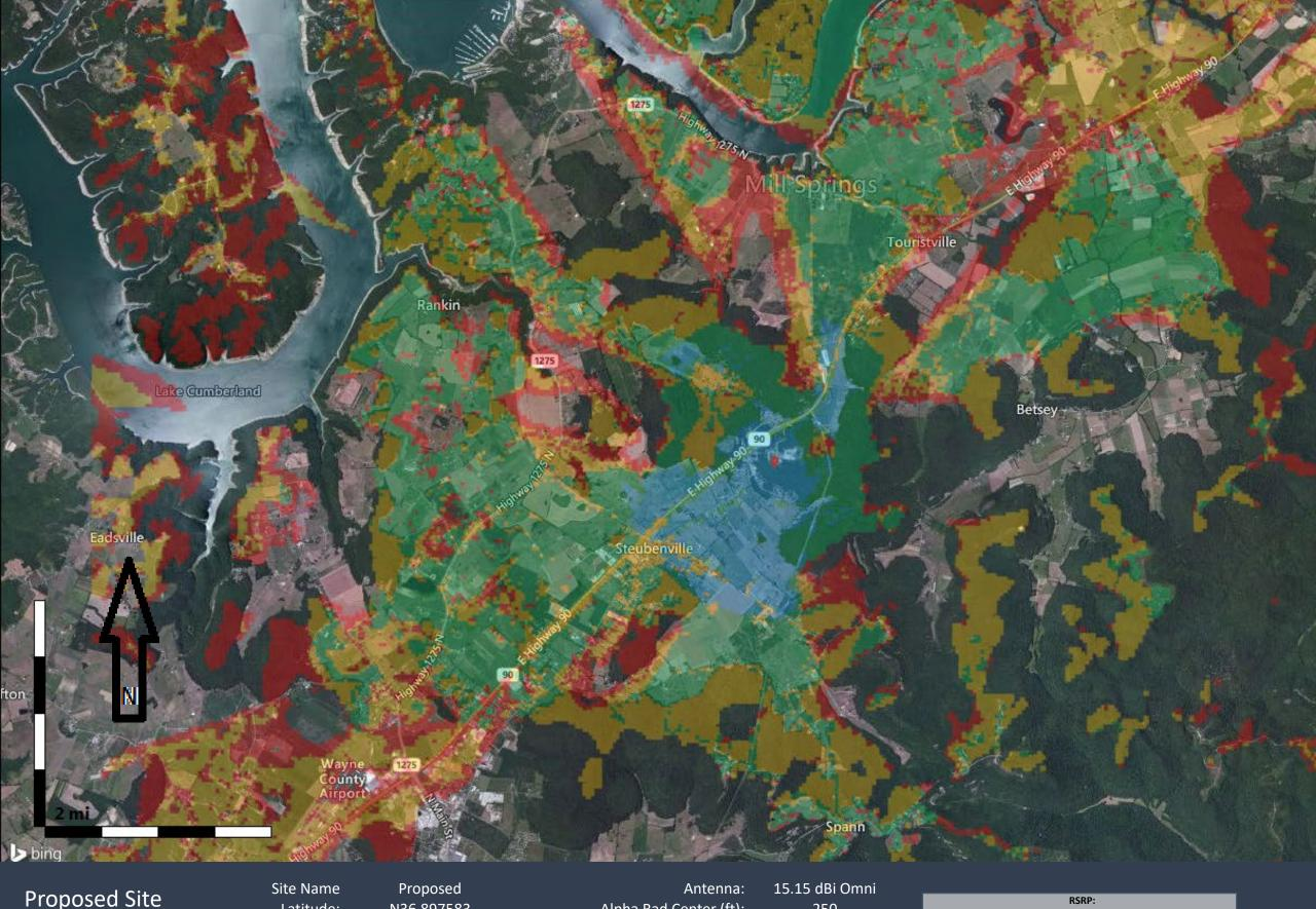
Proposed Site 700 MHz Coverage Site Name Latitude: Longitude: Proposed N36.897583 W84.784972 Antenna: 15.15 dBi Omi Alpha Rad Center (ft): 250 Azimuth (Deg): 0 ERP per RS (W): 2.0
