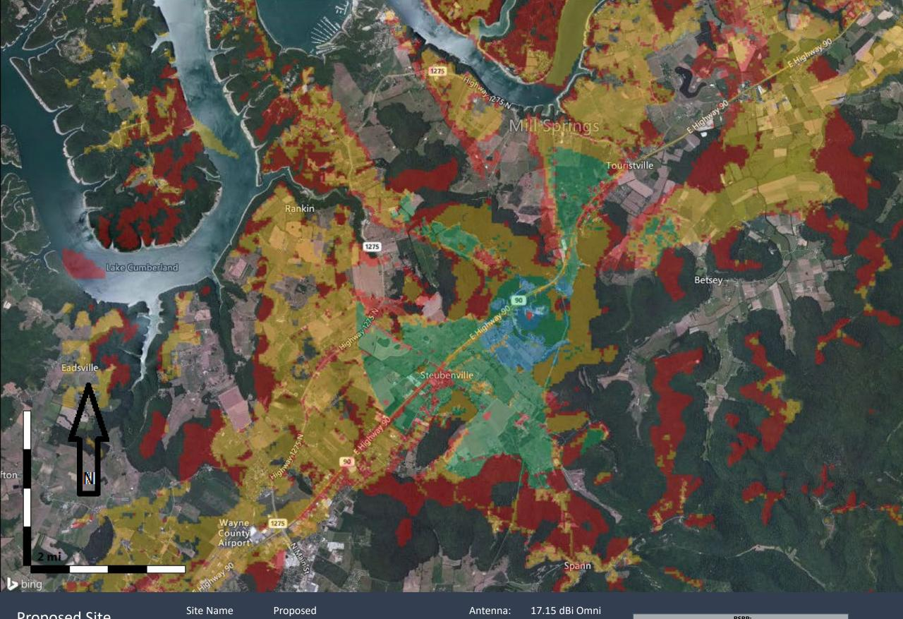
Proposed Site 2100 MHz Coverage Site Name Latitude: Longitude: Proposed N36.897583 W84.784972 Antenna: 17.15 dBi On Alpha Rad Center (ft): 250 Azimuth (Deg): 0 ERP per RS (W): 4.7
