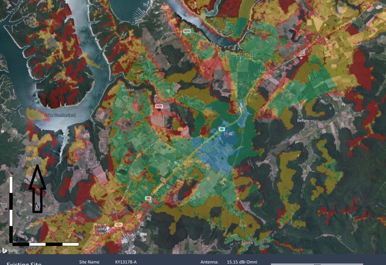
Existing Site 850 MHz Coverage Site Name Latitude: Longitude: KY13178-A N36.897806 W84.784028 Antenna: 15.15 dBi Omr Alpha Rad Center (ft): 240 Azimuth (Deg): 0 ERP per RS (W): 2.0
