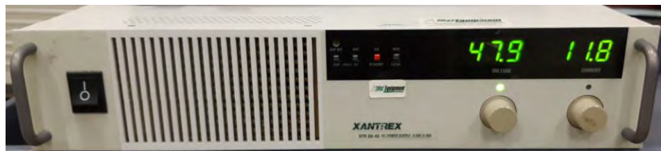
DC power supply for fans
