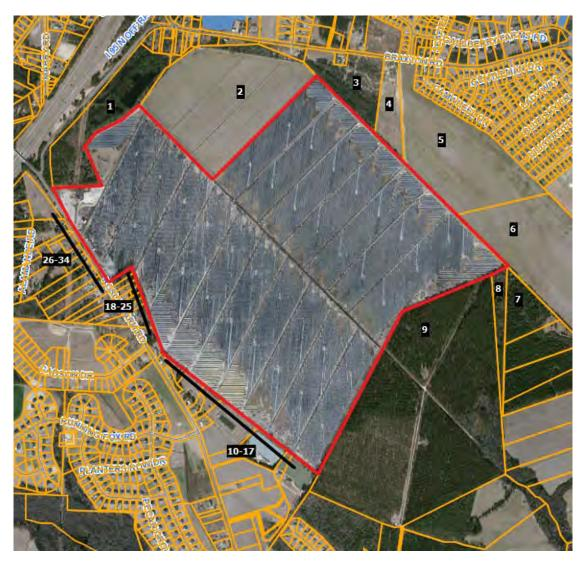
This project was built in 2016 and located on 532 acres for a 78.5 MW solar farm with the closest home at 125 feet from the closest solar panel with an average distance of 423 feet.
