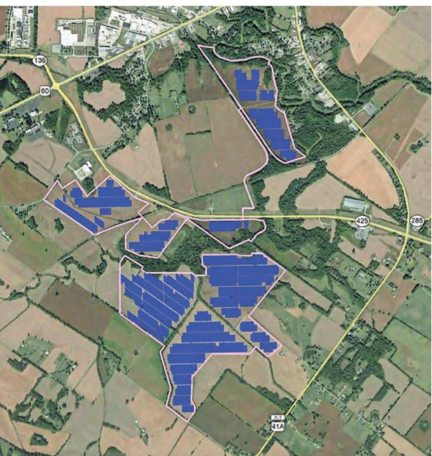
This map shows the planned location of a 514-acre solar farm to be located along the Kentucky 425/South Bypass just outside the Henderson city limits. Most of the solar panels (marked in blue) will be located on the south side of Kentucky 425, with the remainder to be erected on the west side of Lover's Lane.
