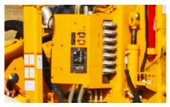
**REDUCE YOUR CYCLE TIME.** Using the auto plumb feature, the PD10 can correct pile angle to be completely vertical without any manual adjustment by the operator. Featuring a hammer which has 80% more impact energy than the original version offered, cycle times have been reduced.
