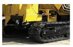
**LEAVE IT LIKE YOU FOUND IT.** The PD10R features a wide track pad to minimize jobsite disturbance in widely varying ground conditions.
