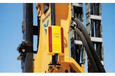
**IMPROVE YOUR ACCURACY.** An optional laser receiver integrated into the control system and a GPS-compatible design (capable of accepting compatible third party systems) can help improve productivity.
