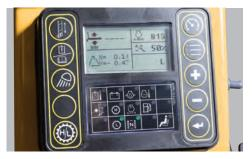
**AT YOUR FINGERTIPS.** An industry-unique integrated control system offers the operator a variety of machine information, including pile angle and height. Display also shows machine maintenance information to help maintain service schedules.
