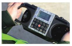
**REMOTE CONTROL.** Control machine functions, including hammer engagement, pile accuracy using the auto plumb feature and ground drive via wireless remote control.
