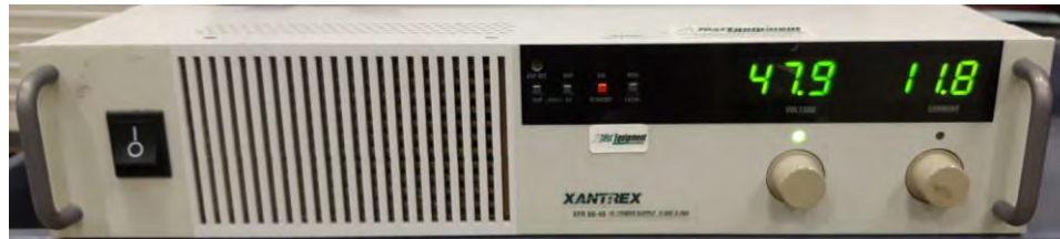
DC power supply for fans
