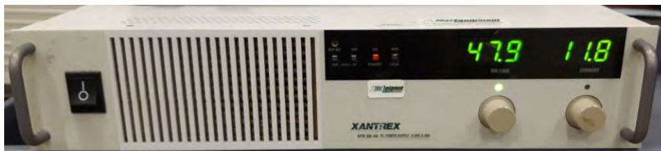
DC power supply for fans
