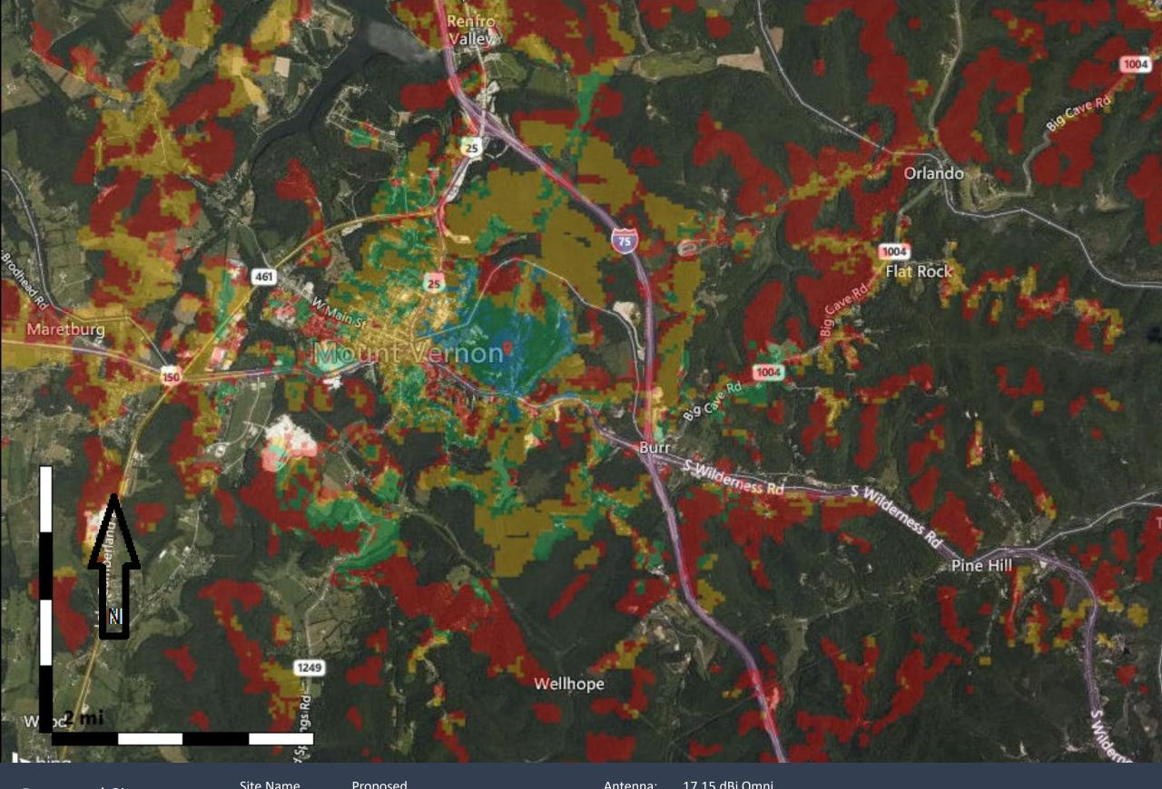
Proposed Site 2100 MHz Coverage Site Name Latitude: Longitude: Proposed N37.35325 W84.327306 Antenna: 17.15 dBi Omni
