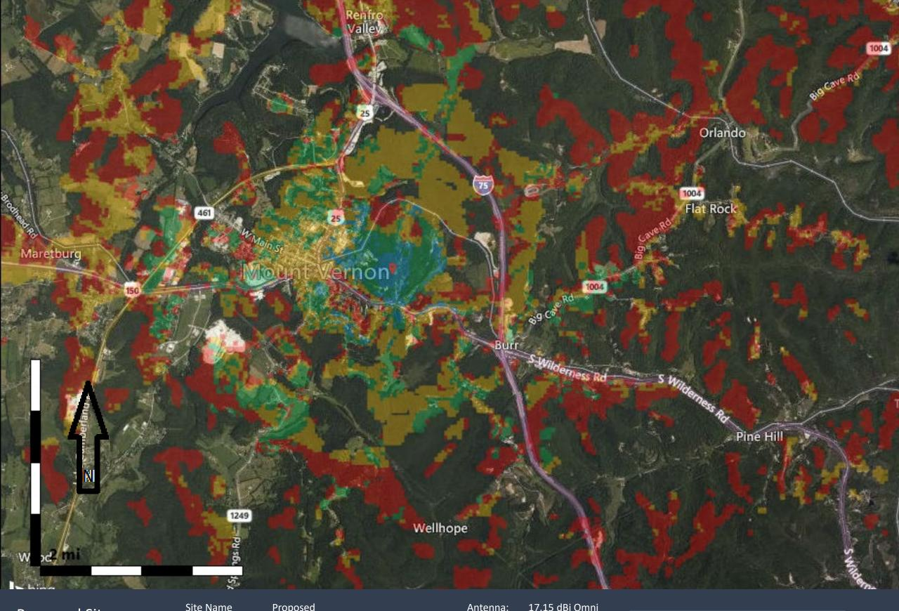
Proposed Site 1900 MHz Coverage Site Name Latitude: Longitude: Proposed N37.35325 W84.327306 Antenna: 17.15 dBi Omni
