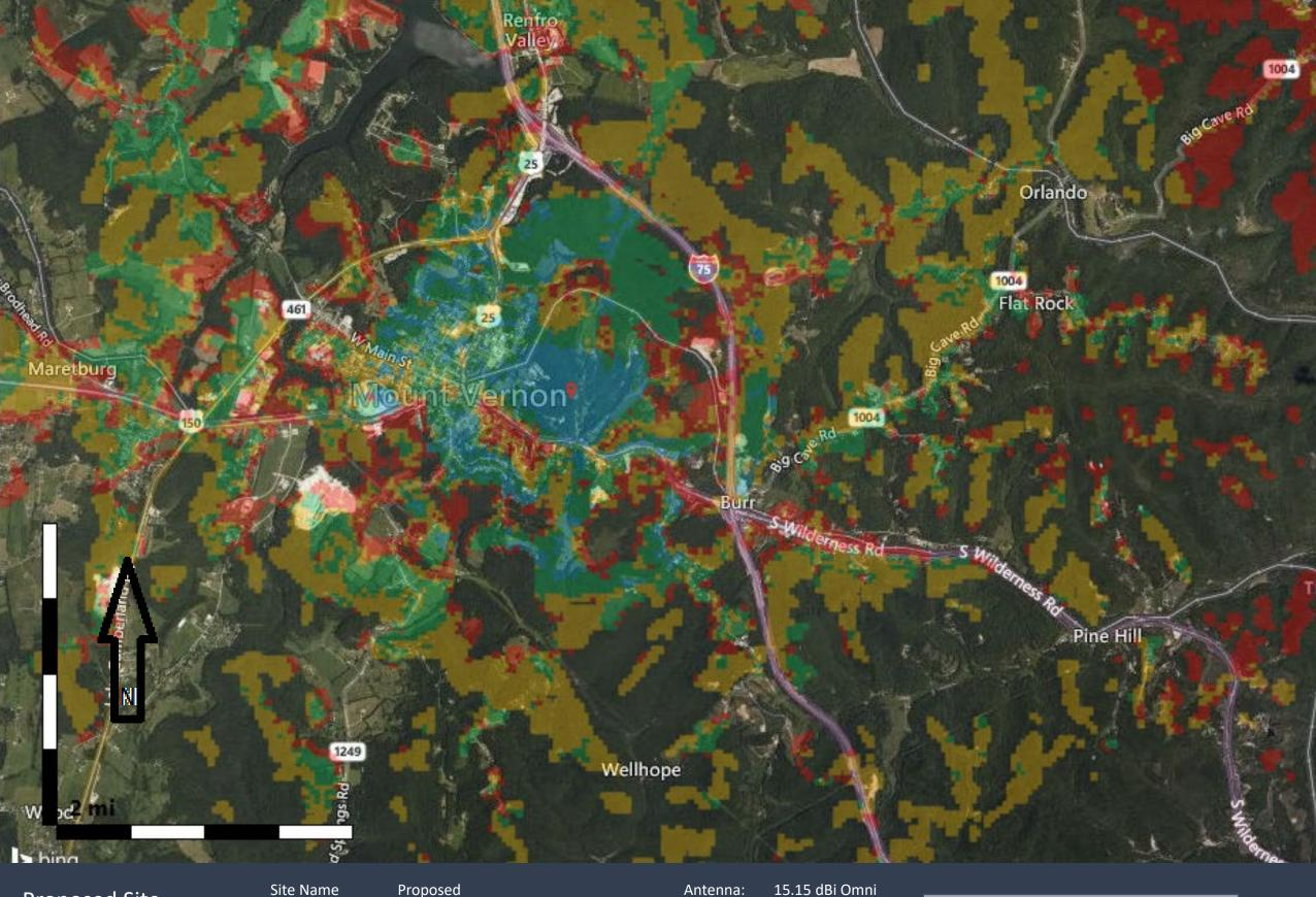
Proposed Site 700 MHz Coverage Site Name Latitude: Longitude: Proposed N37.35325 W84.327306 Antenna: 15.15 dBi Omr Alpha Rad Center (ft): 325 Azimuth (Deg): 0 ERP per RS (W): 2.0
