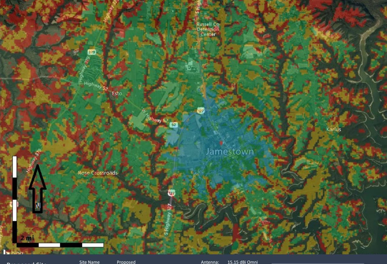
Proposed Site 700 MHz Coverage Site Name Latitude: Longitude: Proposed N36.987586 W85.067219 Antenna: 15.15 dBi Omni
