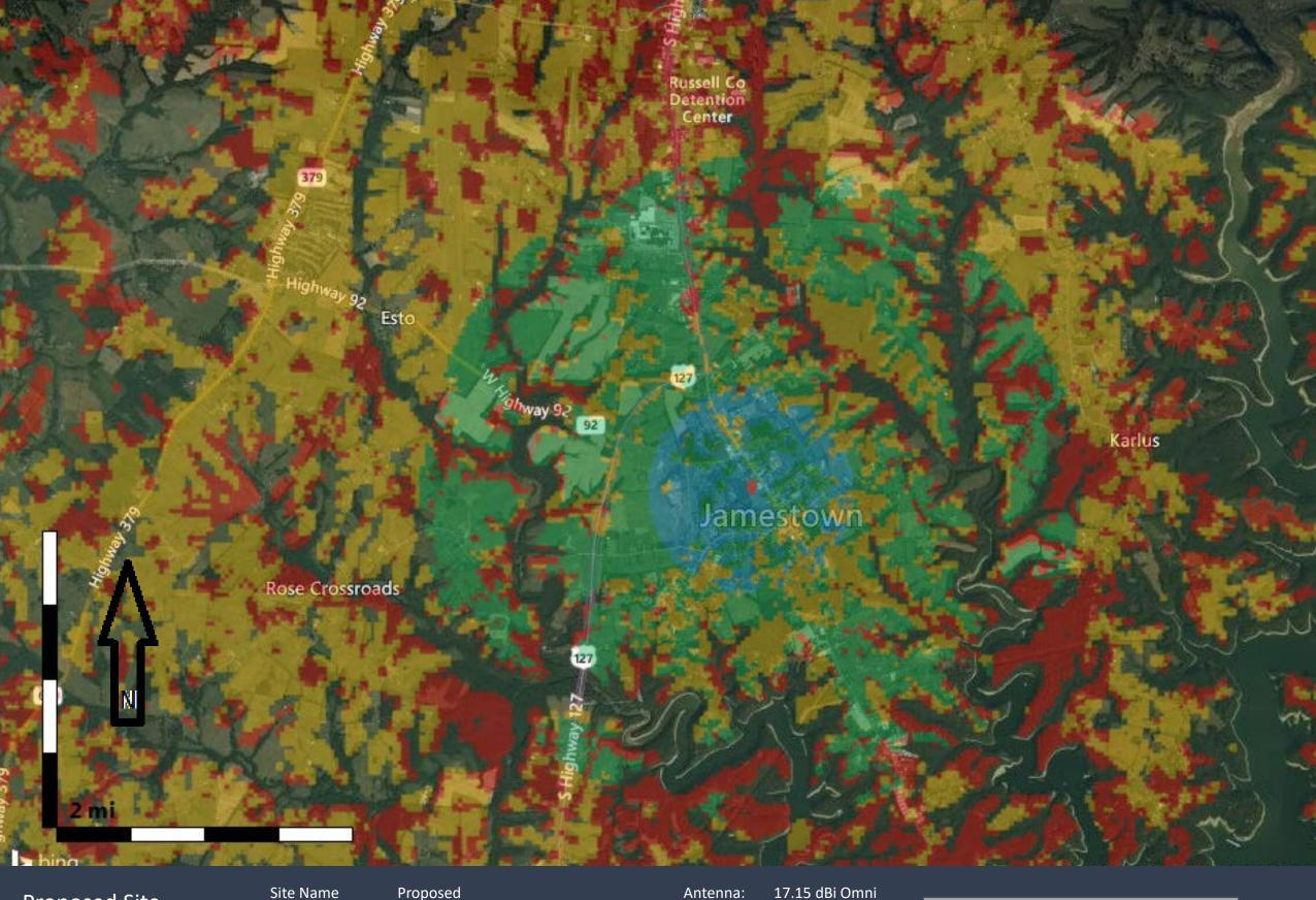
Proposed Site 2100 MHz Coverage Site Name Latitude: Longitude: Proposed N36.987586 W85.067219 Antenna: 17.15 dBi C Alpha Rad Center (ft): 203 Azimuth (Deg): 0 ERP per RS (W): 4.7
