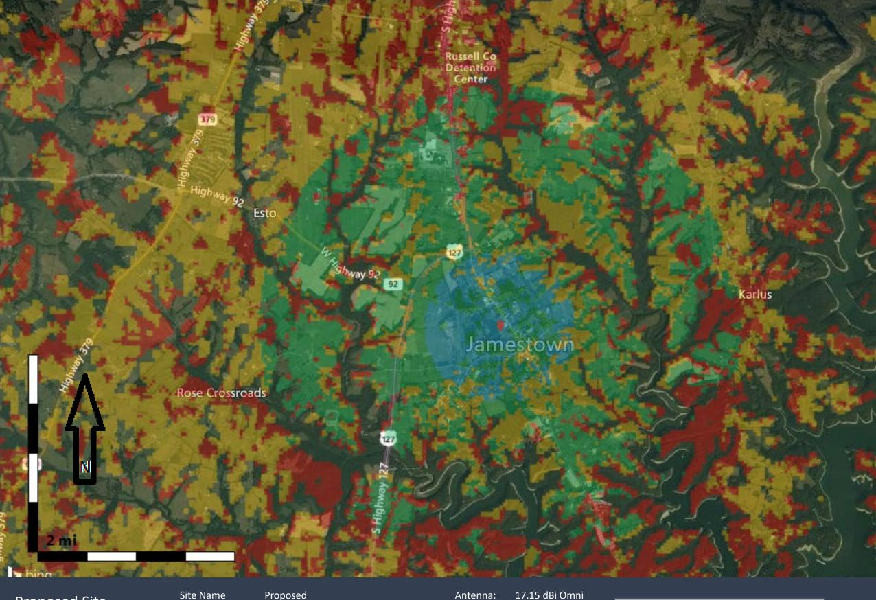
Proposed Site 1900 MHz Coverage Site Name Latitude: Longitude: Proposed N36.987586 W85.067219 Antenna: 17.15 dBi On Alpha Rad Center (ft): 203 Azimuth (Deg): 0 ERP per RS (W): 4.7
