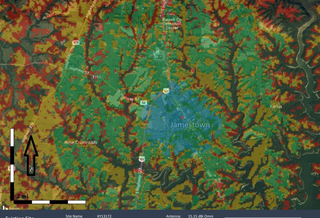
Existing Site 850 MHz Coverage Site Name Latitude: Longitude: KY13172 N36.987483 W85.067497 Antenna: 15.15 dBi Omr Alpha Rad Center (ft): 237 Azimuth (Deg): 0 ERP per RS (W): 2.0
