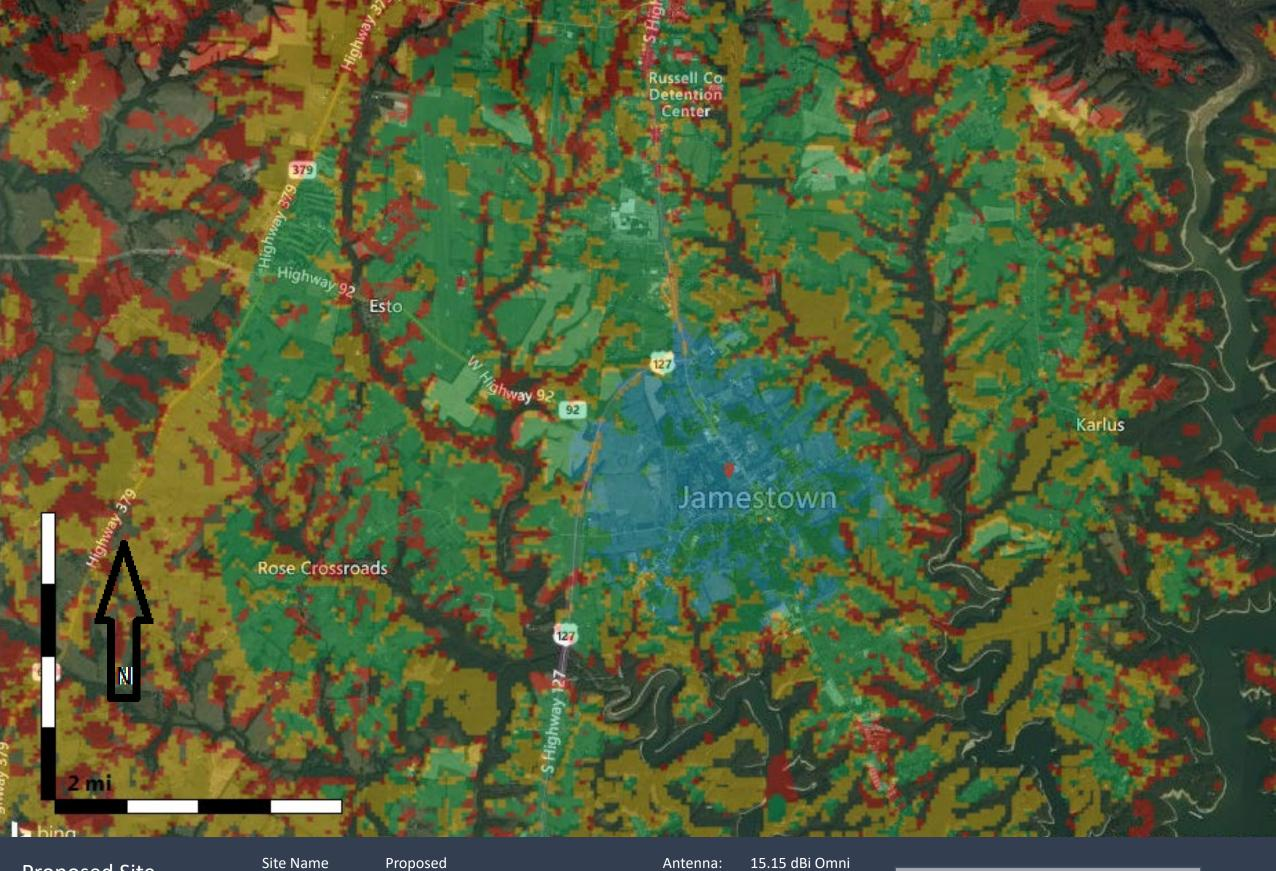
Proposed Site 850 MHz Coverage Site Name Latitude: Longitude: Proposed N36.987586 W85.067219 Antenna: 15.15 dBi Om Alpha Rad Center (ft): 203 Azimuth (Deg): 0 ERP per RS (W): 2.0
