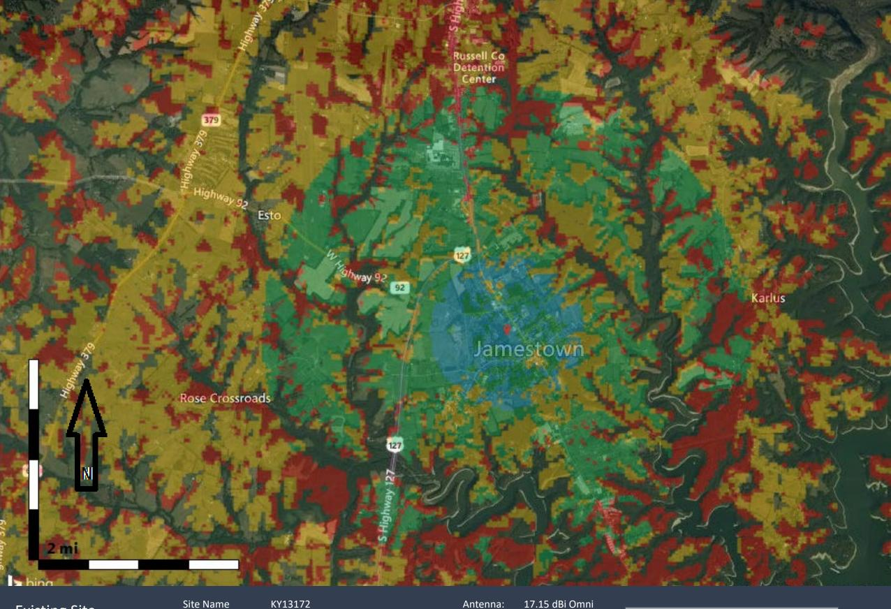
Existing Site 1900 MHz Coverage Site Name Latitude: Longitude: KY13172 N36.987483 W85.067497 Antenna: 17.15 dBi Om Alpha Rad Center (ft): 237 Azimuth (Deg): 0 ERP per RS (W): 4.7
