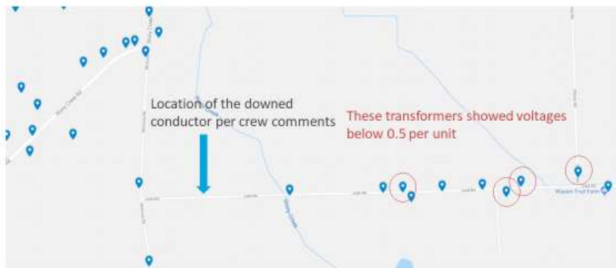
Figure 1-8 Outage event on three-phase delta system
