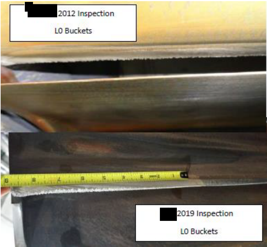
Figure 1. Comparison of bucket leading edge erosion from 2012 to 2019
