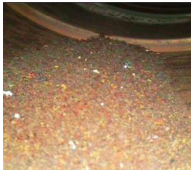
Industry photos of leaking Kettle Boilers and corrosion debris in rotor cooling air piping from ██████████ service bulletin.
