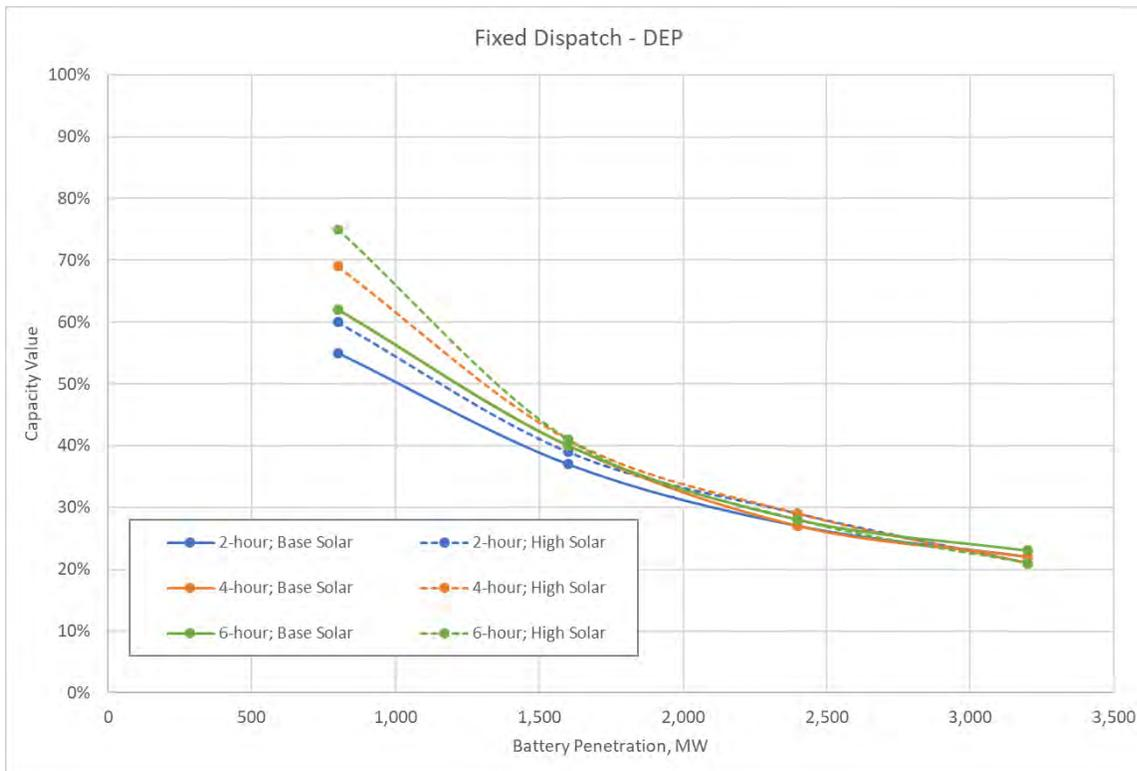
The results of the sensitivity of 6-hour storage added after 3,200 MW of 4-hour storage are shown in the following chart.
