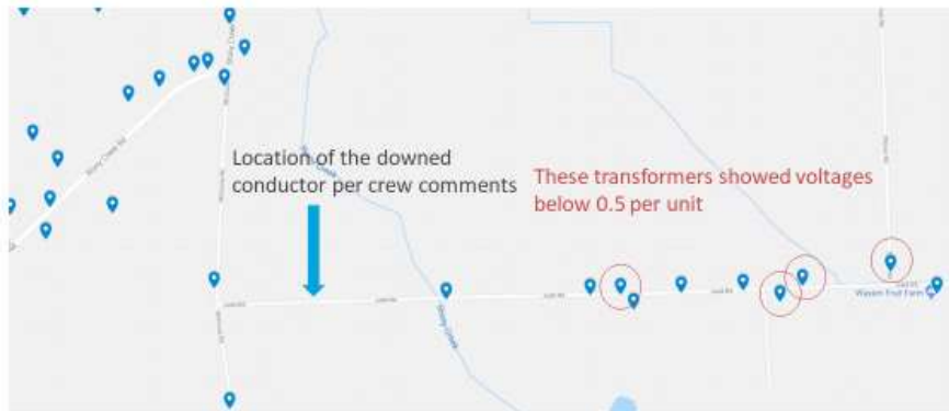
Figure 1-8 Outage event on three-phase delta system
