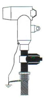
FCI mounted below Loadbreak Elbow
