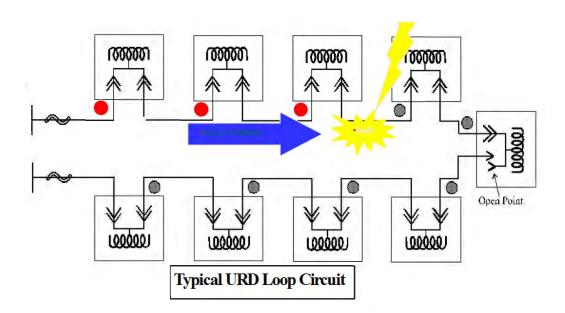
By switching out the faulted segment, power can be restored to the balance of the circuit while the faulted segment is repaired. FCl's can be used for troubleshooting or can be permanently left in place on the circuit. Reducing the duration of the outage can lead to improvements in reliability indices such as SAIDI and CAIDI.
