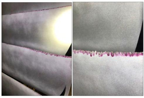
Figure 2. Leading edge erosion in 2019
