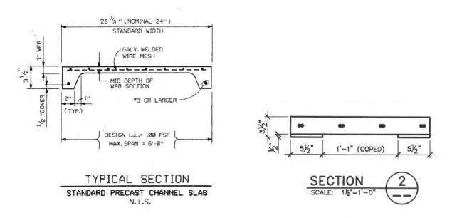
Figure 2. Cross-section of typical existing floor panel.
