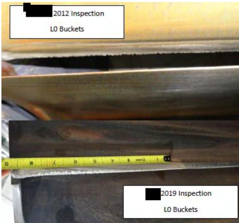
Figure 1. Comparison of bucket leading edge erosion from 2012 to 2019
