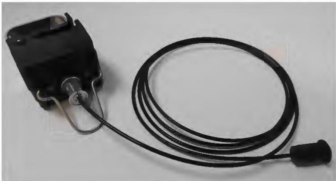
FCI Load Tracker LM with Fiber Optic Remote Indication
