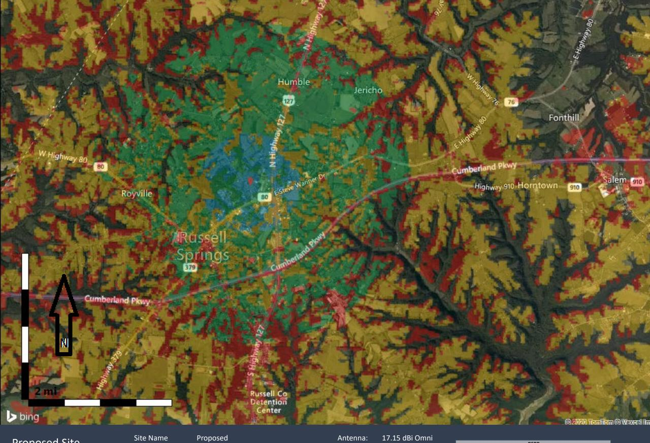
Proposed Site 2100 MHz Coverage Site Name Latitude: Longitude: Proposed N37.068689 W85.077047 Antenna: 17.15 dBi Omn Alpha Rad Center (ft): 225 Azimuth (Deg): 0 ERP per RS (W): 4.7
