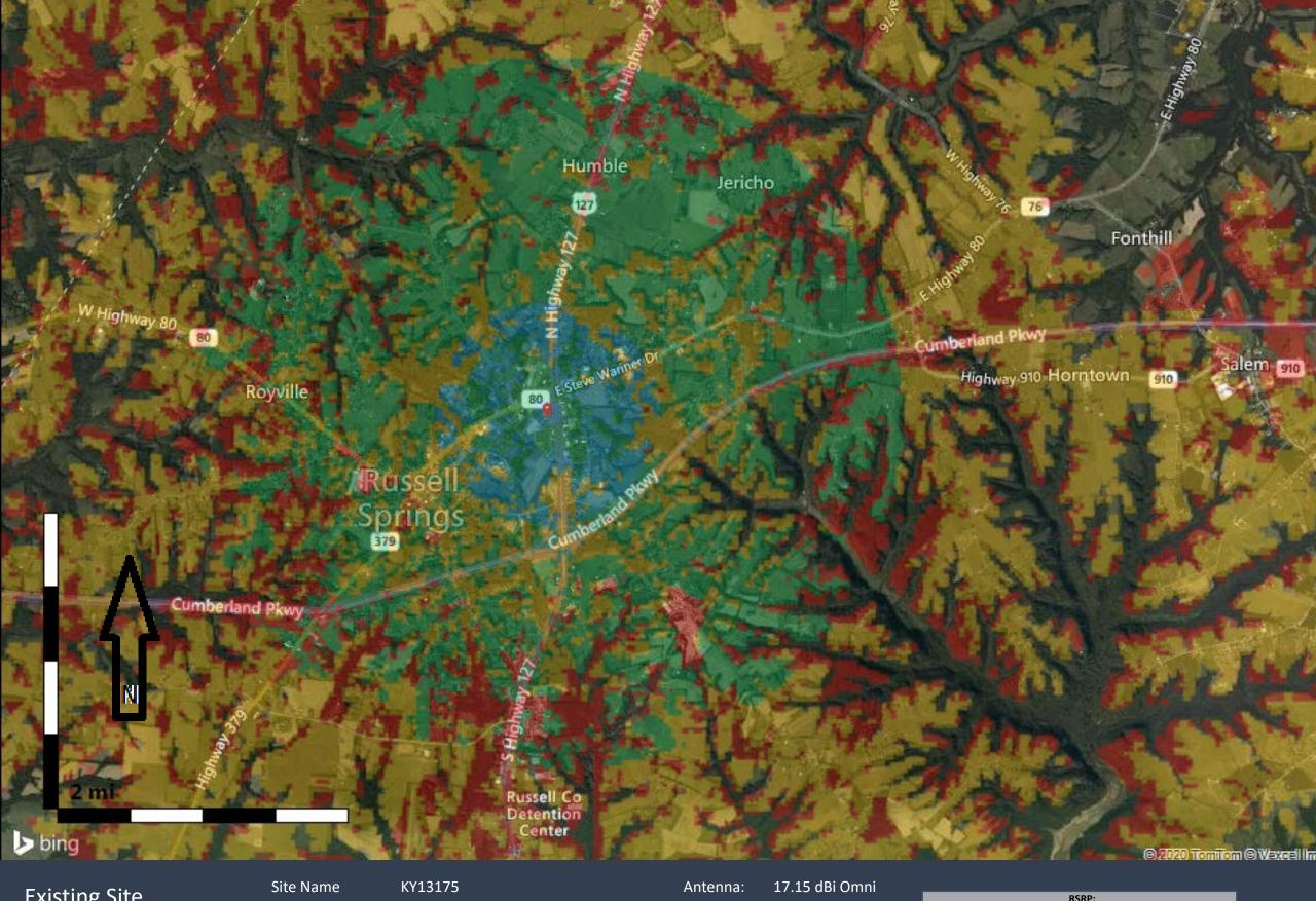
Existing Site 1900 MHz Coverage Site Name Latitude: Longitude: KY13175 N37.064417 W85.072083 Antenna: 17.15 dBi Om Alpha Rad Center (ft): 230 Azimuth (Deg): 0 ERP per RS (W): 4.7
