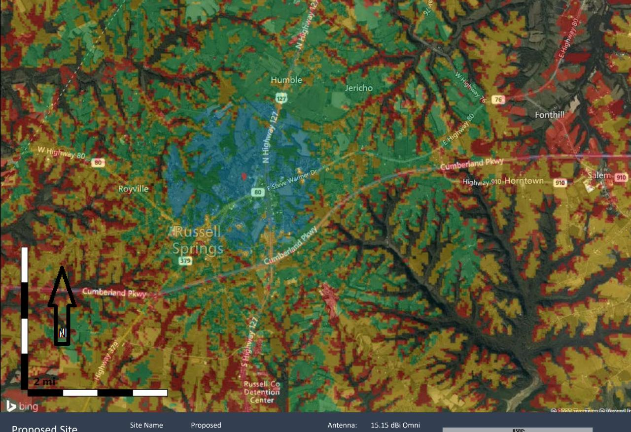
Proposed Site 850 MHz Coverage Site Name Latitude: Longitude: Proposed N37.068689 W85.077047 Antenna: 15.15 dBi
