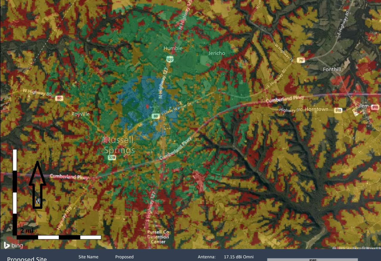
Proposed Site 1900 MHz Coverage Site Name Latitude: Longitude: Proposed N37.068689 W85.077047 Antenna: 17.15 dBi C Alpha Rad Center (ft): 225 Azimuth (Deg): 0 ERP per RS (W): 4.7
