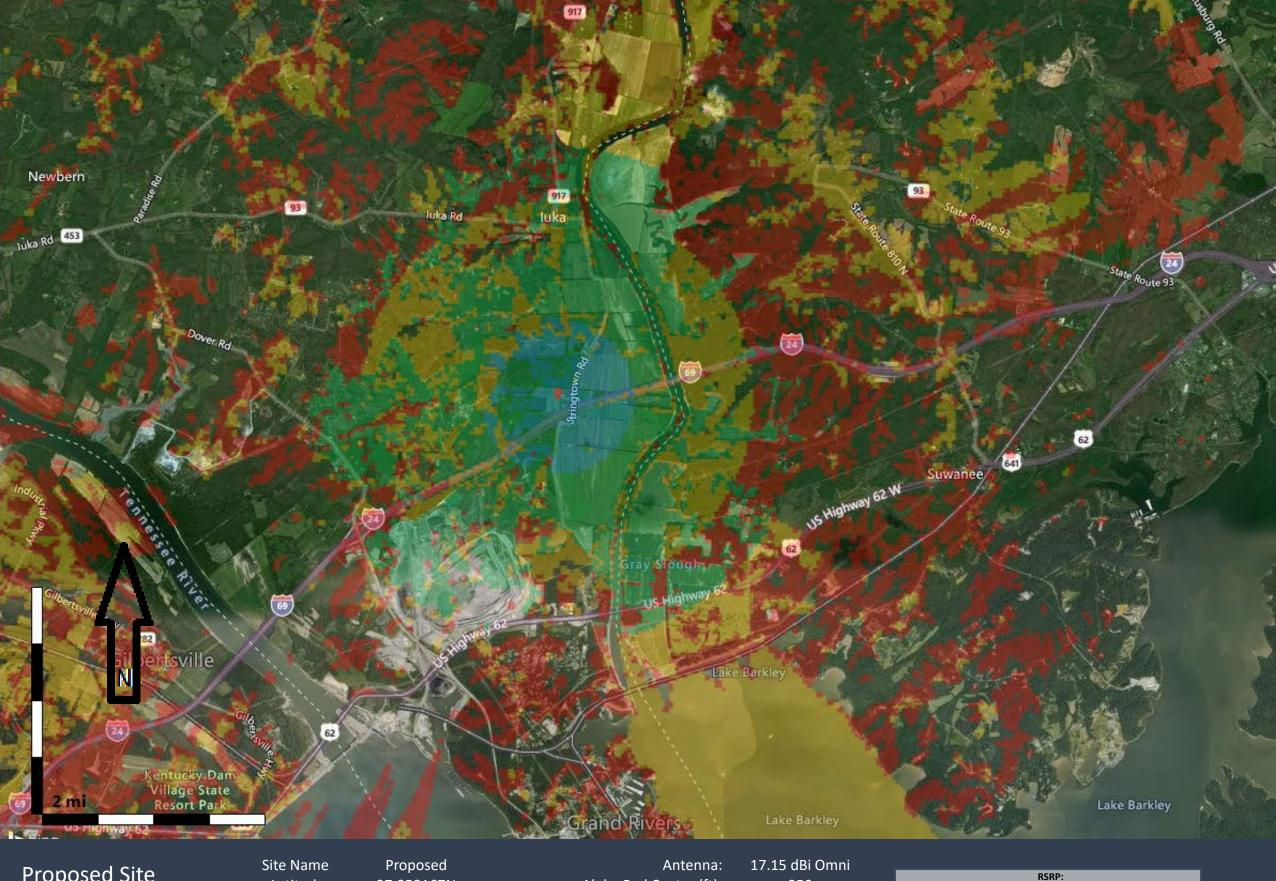
Proposed Site 2100 MHz Coverage Site Name Latitude: Longitude: Proposed 37.058167N 88.236361W Antenna: 17.15 dBi Omr Alpha Rad Center (ft): 250 Azimuth (Deg): 0 ERP per RS (W): 4.7
