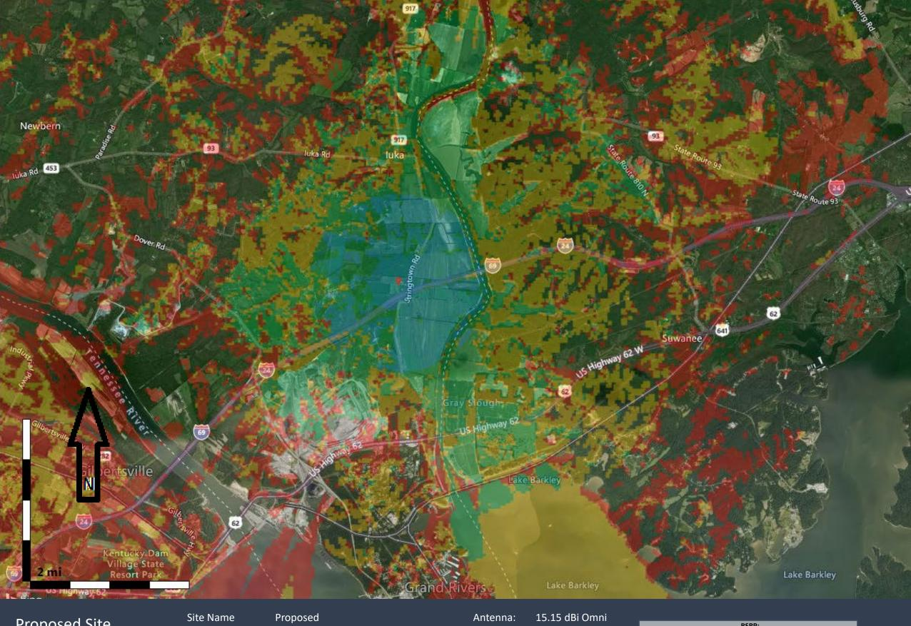
Proposed Site 850 MHz Coverage Site Name Latitude: Longitude: Proposed 37.058167N 88.236361W Antenna: 15.15 dBi Omn Alpha Rad Center (ft): 250 Azimuth (Deg): 0 ERP per RS (W): 2.0
