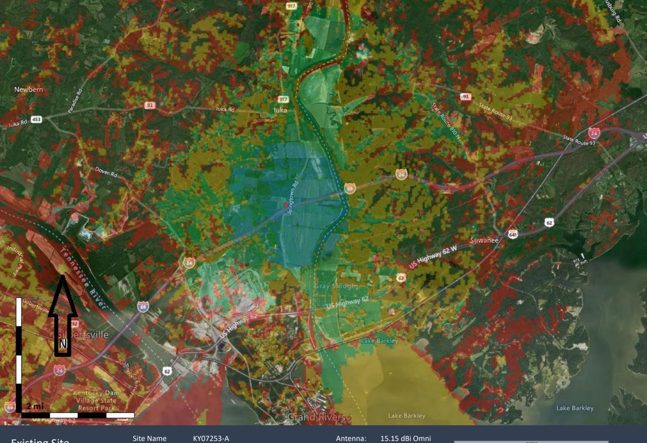
Existing Site 850 MHz Coverage Site Name Latitude: Longitude: KY07253-A 37.056819N 88.235364W Antenna: 15.15 dBi Omni Alpha Rad Center (ft): 250 Azimuth (Deg): 0 ERP per RS (W): 2.0
