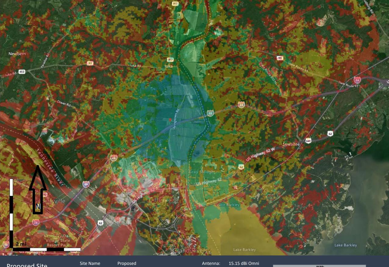
Proposed Site 700 MHz Coverage Site Name Latitude: Longitude: Proposed 37.058167N 88.236361W Antenna: 15.15 dBi Omni Alpha Rad Center (ft): 250 Azimuth (Deg): 0 ERP per RS (W): 2.0
